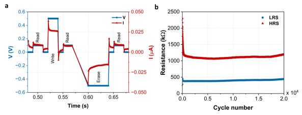
Fig. 9 Resistive switching properties; (a) measurement of change in conductance state during a resistive switching cycle in an IL-functionalized GP memristor. There is a read pulse of 0.1 V, 20 ms between the write pulse (0.5 V, 20 ms) and the erase pulse (-0.5 V, 50 ms) which completes a full acquisition; (b) the cycle in a was repeated over 20 000 times demonstrating retention window of IL-functionalized GP memristors over 20 000 cycles with reading voltage of 100 mV.
