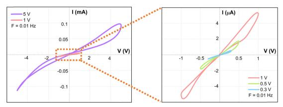
Fig. 5 I-V plot of an IL-functionalized geopolymer sample ( $\phi=1000~\mu m$ ) under different sinusoidal waveforms and a constant frequency of 0.01 Hz.
