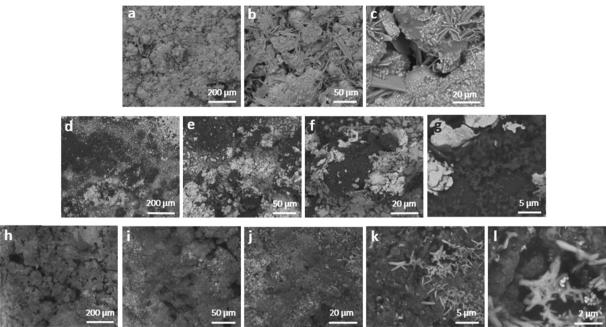
Fig. 6 (a)-(c) SEM images of IL-functionalized geopolymer samples without silver adhesive to show the natural interaction between the geopolymer and EMIM+ Otf-; (d)-(g) SEM images of IL-functionalized geopolymer samples including a layer of silver adhesive on them before testing; and (h)-(l) SEM images of IL-functionalized geopolymer samples after testing. ( $\phi = 1000 \mu m$  and  $h = 140 \mu m$  for all the samples).
