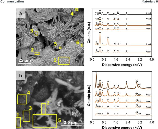
EDX spectra of the IL-functionalized geopolymer (a) without silver adhesive applied, and (b) after testing.
