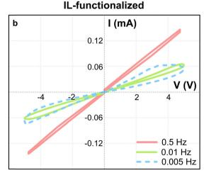
Fig. 2 /-V graphs under sinusoidal waveforms at varying frequencies (0.005 Hz, 0.01 Hz, and 0.5 Hz) for (a) pristine and (b) IL-functionalized GP devices. All tests were conducted on devices with  $\phi$  = 1000  $\mu$ m.
