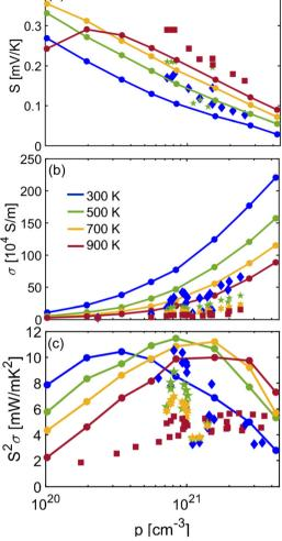
Fig. 8 Comparison with experimental values: our calculations for: (a) Seebeck coefficient, (b) electrical conductivity, and (c) power factor for p-type NbFeSb *versus* doping concentration for various temperatures. The diamond, star, hexagram, and square markers correspond to experimentally reported values from ref. 23 and 27–34.
