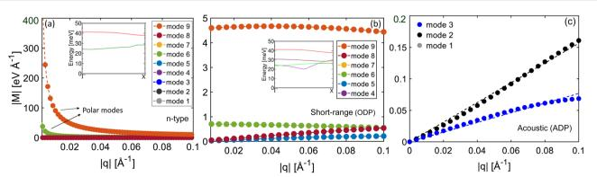
Fig. 4 Scattering matrix elements for intravalley deformation potential exaction for electrons: (a) for all phonons (two modes show polar behaviour) along the  $\Gamma$ -X direction. (b) Short range part of matrix elements for optical and (c) acoustic phonons for scattering from the conduction band minima (CBM to CBM). The insets in (a) and (b) show the frequencies corresponding to the polar optical and non-polar optical modes, respectively.
