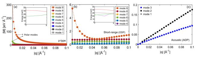
Fig. 2 Scattering matrix elements for intravalley deformation potential extraction for holes: (a) for all phonons (two modes show polar behaviour) along the  $\Gamma$ -X direction. (b) Short range part of the matrix elements for optical and (c) acoustic phonons for scattering from the valence band maxima (VBM to VBM). The insets in (a) and (b) show the frequencies corresponding to the polar optical and non-polar optical modes, respectively
