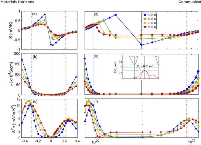
Fig. 7 Electronic transport properties: (a) calculated Seebeck coefficient, (b) electrical conductivity and (c) power-factor versus the Fermi level position E<sub>F</sub> (left-panel) and (d-f) versus the doping density (right-panel). Here we consider all relevant scattering mechanisms (ADP, ODP, POP, IIS). The blue and red dashed lines show the band edges and the black line shows the intrinsic fermi level.
