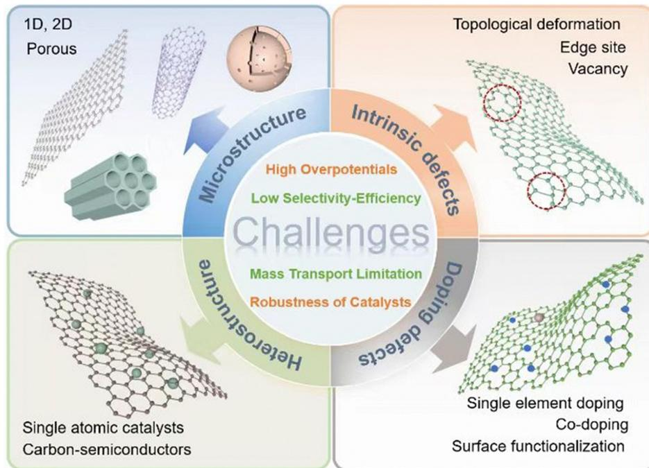
Fig. 1 Schematics of key challenges and corresponding modification strategies of carbon-based electrocatalysts for  $\text{H}_2\text{O}_2$  production.
