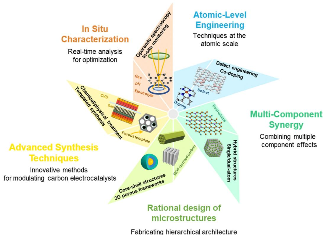
Fig. 17 Schematic of perspective strategies for rational design of carbon catalysts (atomic level engineering, multiple-synergistic effects), advanced synthesis method, and *in situ* characterization techniques.
