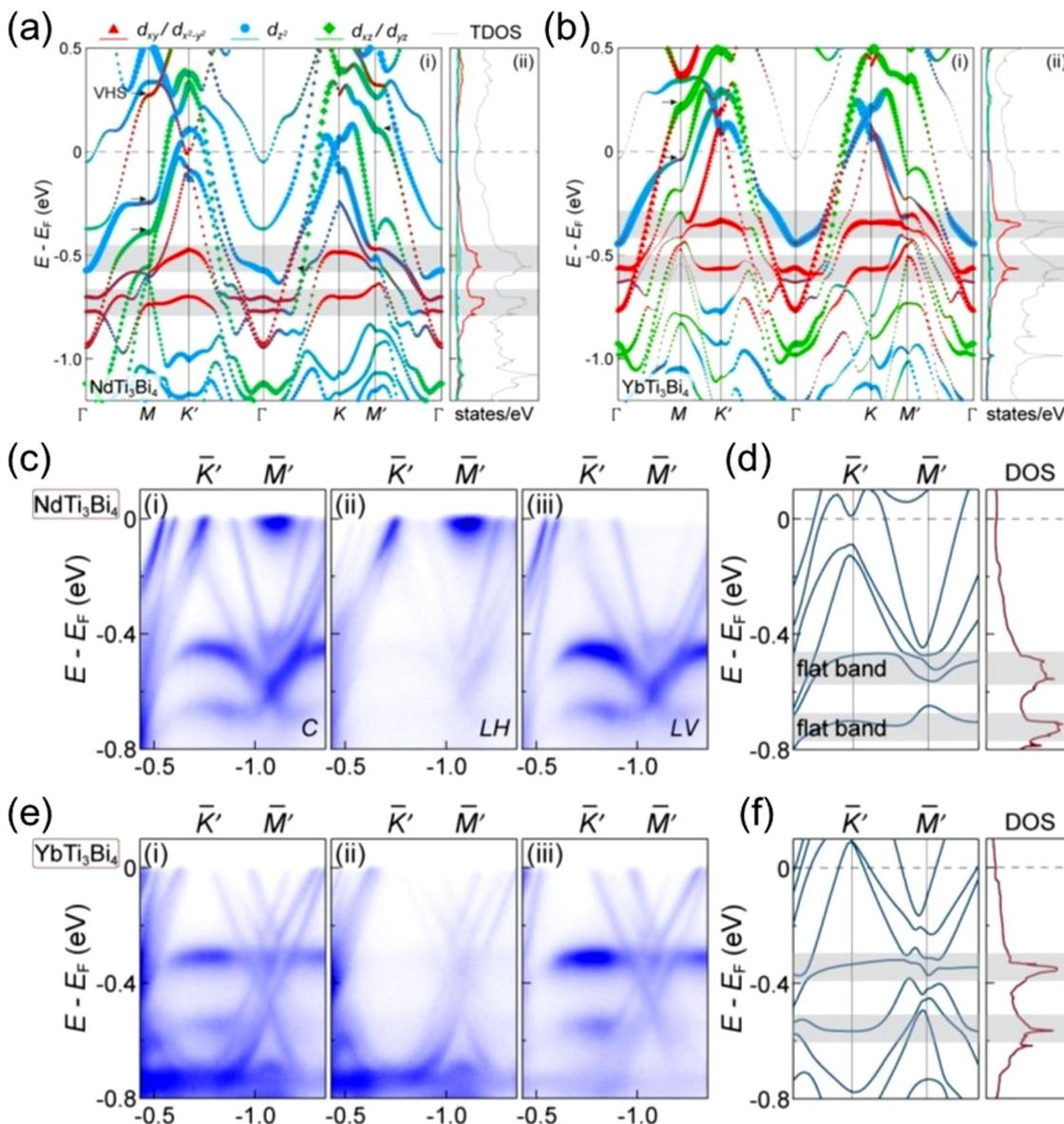
Fig. 8 Orbital resolved electronic band structures of (a)  $\text{NdTi}_3\text{Bi}_4$  and (b)  $\text{YbTi}_3\text{Bi}_4$ . Experimental band dispersions of (c)  $\text{NdTi}_3\text{Bi}_4$  and (e)  $\text{YbTi}_3\text{Bi}_4$ . DFT calculated band structure of (d)  $\text{NdTi}_3\text{Bi}_4$  and (f)  $\text{YbTi}_3\text{Bi}_4$ .<sup>50</sup>
