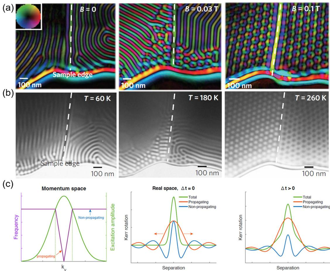
Fig. 13 (a) The variation of the skyrmion lattice with the external magnetic field at  $T = 260$  K and (b) the variation of the skyrmion lattice with the temperature at  $B = 0.1$  T in FeGe.<sup>120</sup> (c) Schematic representation of the fundamental mechanism underlying the formation of wavepacket precursors.<sup>107</sup> (a) and (b) Are reproduced with permission from ref. 120.
