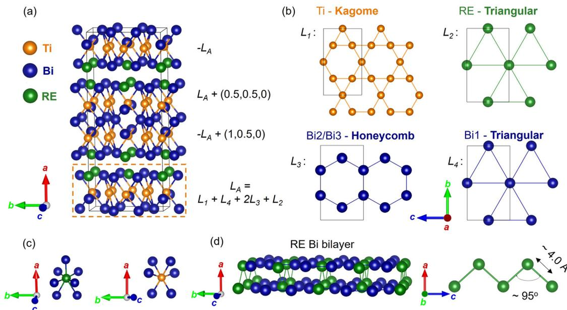
Fig. 3 (a) Crystal structure of  $\text{Ln}(\text{RE})\text{Ti}_3\text{Bi}_4$ . (b) Kagome network of Ti ( $L_1$ ), triangular lattice of RE ( $L_2$ ), honeycomb ( $L_3$ ) and triangular lattice of Bi ( $L_4$ ). (c) The coordination environment of RE and Ti. (d) The REBi bilayer and Ln–Ln zigzag chains.
