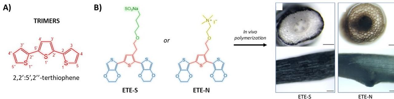
Fig. 9 (A) Chemical structure of terthiophene (thiophene trimer). (B) Chemical structures of ETE-N and ETE-S trimers polymerized *in vivo* along the roots of living plants due to the presence of native peroxidase enzymes, and cross-sectional (top) and lateral views (bottom) of the bean roots (scale bar = 100  $\mu$ m). Adapted and reprinted with permission.<sup>126</sup> Copyright 2020 American Chemical Society.
