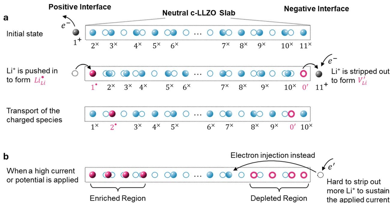
Fig. 3 Schematic explanations of (a) the generation and transport of  $Li_{Li}^{\bullet}$  at the positive interface and  $V'_{Li}$  at the negative interface in a single Li-ion conducting channel, due to the electrochemical transfer of  $Li^+$  ions across the interfaces; and (b) the scenario of the generation and accumulation of  $Li_{Li}^{\bullet}$  and  $V'_{Li}$  in high-current conditions.
