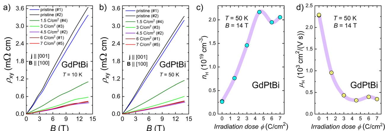
Fig. 2 Magnetic field dependence of Hall electrical resistivity at  $T = 10$  K (a) and  $T = 50$  K (b). Carrier concentration (c) and carrier mobility (d) as a function of irradiation dose at  $T = 50$  K.
