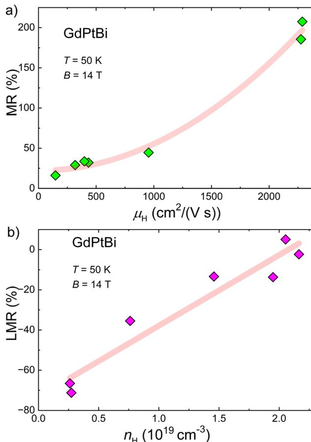
Fig. 4 Transverse (a) and longitudinal (b) magnetoresistance of pristine and electron irradiated samples as a function of carrier mobility (a) and carrier concentration (b) at  $T = 50$  K and under  $B = 14$  T. Pink lines are a guide to the eye.
