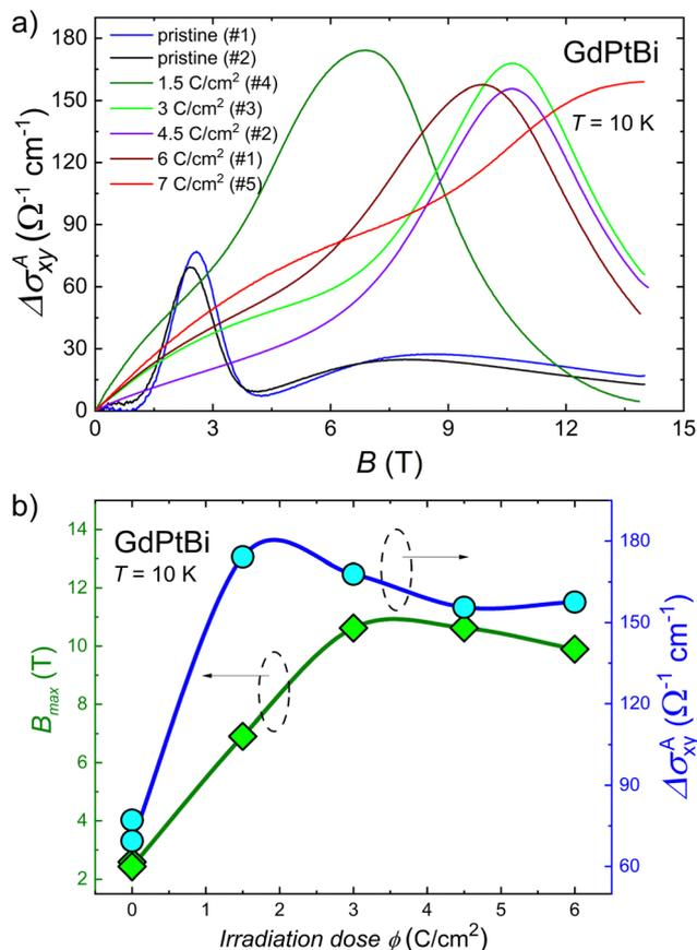
Fig. 5 (a) Anomalous Hall conductivity as a function of magnetic field at  $T = 10$  K for pristine and irradiated samples. (b) Maximum values of anomalous Hall conductivity (right axis) and magnetic field values (left axis) at which these maxima were recorded as a function of irradiation dose at  $T = 10$  K.
