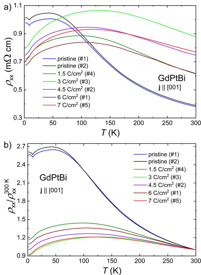
Fig. 1 Temperature dependence of the electrical resistivity (a) and normalised electrical resistivity to the value of  $\rho$  recorded at  $T = 300$  K (b) of pristine and irradiated GdPtBi samples, measured with an electrical current ( $j$ ) applied along the [001] crystallographic direction and in zero magnetic field.
