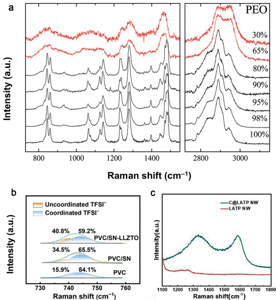
Fig. 20 Raman spectra of (a) PEO and of PEO/Na<sup>+</sup>-MMT nanocomposites with different polymer concentrations at ambient temperature. Reproduced with permission from ref. 148. Copyright 2011, American Chemical Society. (b) PVC, PVC/SN and PVC/SN-LLZTO SEs in the range of 730–760 cm<sup>-1</sup>. Reproduced with permission from ref. 149. Copyright 2024, Wiley-VCH GmbH. (c) The C@LATP NW and LATP NW. Reproduced with permission from ref. 116. Copyright 2024, Royal Society of Chemistry.
