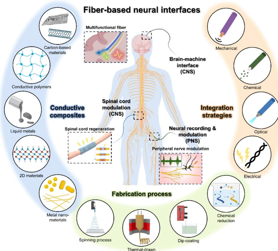
Fig. 1 Introduction of emerging fiber-based neural interfaces.
