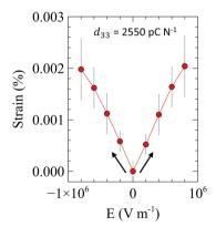
**Fig. 6** Longitudinal piezoelectric measurement on a sample of PMN-33PT cycled  $\sim$ 20 times. The slope was averaged between the negative and positive fields to obtain a  $d_{33}$  value of 2550 pC N $^{-1}$  for the cycled sample.
