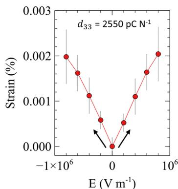
Fig. 6 Longitudinal piezoelectric measurement on a sample of PMN-33PT cycled  $\sim 20$  times. The slope was averaged between the negative and positive fields to obtain a  $d_{33}$  value of  $2550 \text{ pC N}^{-1}$  for the cycled sample.
