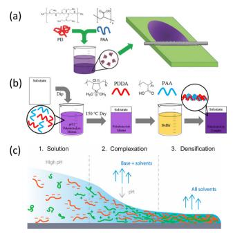
Fig. 5 Examples of PEC coacervate/solution-deposited coatings: (a) PEI/ PAA coacervate oxygen barrier coatings. Reproduced with permission. 126 Copyright 2017, Wiley-VCH. (b) PDADMAC/PAA solution oxygen barrier coatings, reproduced with permission. 128 Copyright 2018, American Chemical Society. (c) Film formation mechanism of evaporation-induced complexation coatings. Green: PEI, orange: polyanion, reproduced with permission. 133 Copyright 2024, American Chemical Society.
