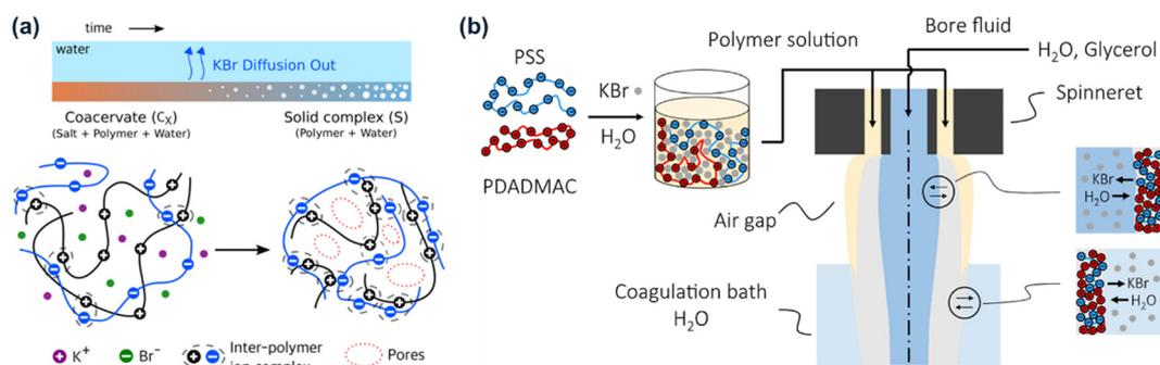
Fig. 4 Schematic illustration of PEC-based (a) flat membranes (reproduced with permission.<sup>98</sup> Copyright 2019, American Chemical Society) and (b) hollow-fiber membranes (reproduced with permission.<sup>101</sup> Copyright 2021, Wiley) *via* salinity change-induced APS.
