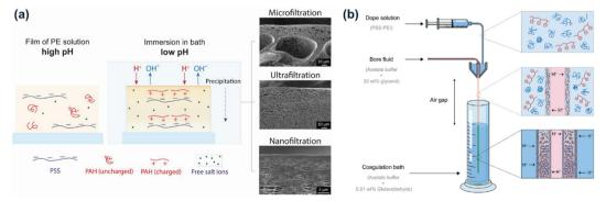
Fig. 3 Schematic illustration of PEC-based (a) flat membranes (reproduced with permission.<sup>89</sup> Copyright 2020, Wiley) and (b) hollow-fiber membranes (reproduced with permission.<sup>94</sup> Copyright 2022, American Chemical Society) via pH change-induced APS.
