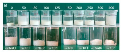
Fig. 9 (a) Effect of NaCl concentration (0–400 mM) on PSS-PDADAMC PEC formation. (b) and (c) Effect of salt type and salt concentration [(b) 125 mM and (c) 250 mM] on PSS-PDADMAC PEC formation – from Krishna et al.<sup>211</sup>
