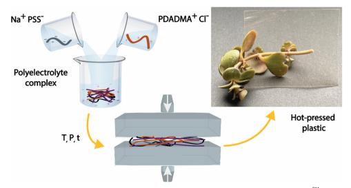
Fig. 10 Schematic of hot-pressing polyelectrolyte complexes into dense saloplastic membranes – from Krishna et al. 211
