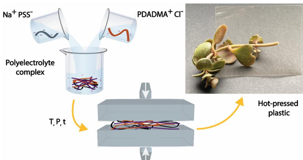
Fig. 10 Schematic of hot-pressing polyelectrolyte complexes into dense saloplastic membranes – from Krishna *et al.*<sup>211</sup>
