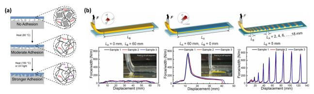
Fig. 7 Enhancement of adhesion strength. (a) Schematic illustration of enhancing surface wetting based on temperature and UV irradiation.<sup>89</sup> Copyright 2016, American Chemical Society. (b) Peel strength for soft and stiff segments. 33 Copyright 2024, Elsevier.
