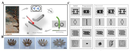
Fig. 8 4D printing of lignin materials. (A) Lignin as a photothermal module for shape memory composites. <sup>71</sup> Copyright 2023, Elsevier. (B) The shape recovery process of 3D-printed petals at different UV irradiation times (0-10 min). Under UV light, the petals change from buds to flowers. 161 Copyright 2023, Elsevier. (C) Shape memory for 3D printing different structures in a water bath at 70 °C. 71 Copyright 2023, Elsevier.
