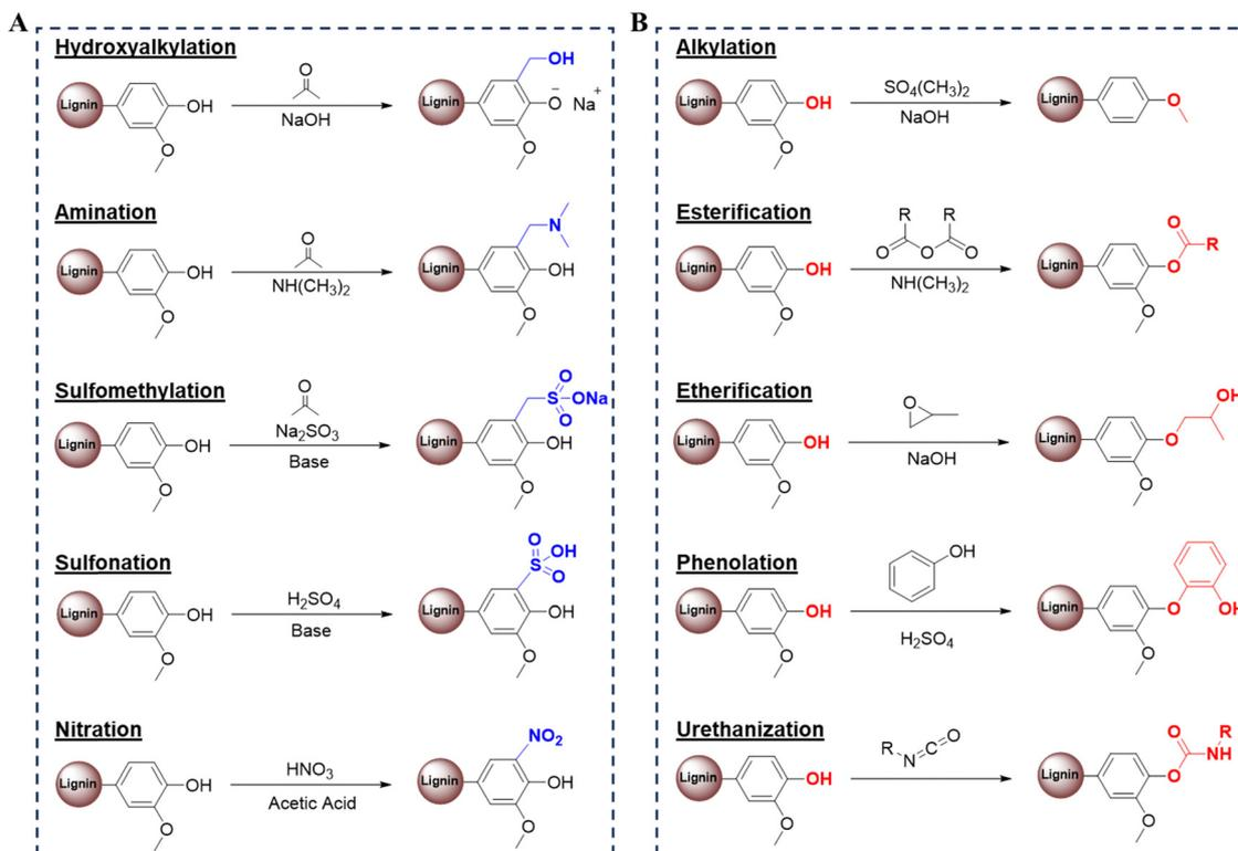
Fig. 2 (A) Schematic overview of chemical modifications generating new active sites in lignin and (B) schematic overview illustrating the functionalization of lignin's hydroxyl groups.<sup>32</sup> Copyright 2019, Elsevier.
