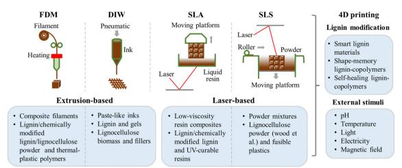
Fig. 3 Scheme of different 3D printing techniques used for lignin-based materials and derived 4D printing of lignin materials. Material extrusion: FDM and DIW; laser-based: SLA and SLS.
