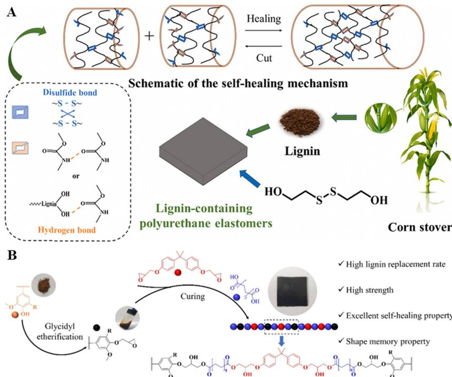
Fig. 7 (A) Schematic overview of lignin-based PU with self-healing properties.<sup>152</sup> Copyright 2021, Elsevier. (B) Schematic overview of the development of a lignin-based vitrimer as a sustainable alternative to bisphenol A epoxy resin.<sup>154</sup> Copyright 2021, Elsevier.
