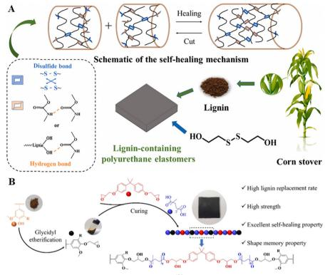
Fig. 7 (A) Schematic overview of lignin-based PU with self-healing properties. <sup>152</sup> Copyright 2021, Elsevier. (B) Schematic overview of the development of a lignin-based vitrimer as a sustainable alternative to bisphenol A epoxy resin. <sup>154</sup> Copyright 2021, Elsevier.
