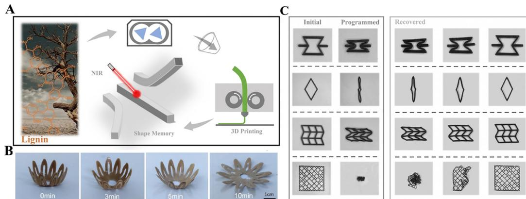
Fig. 8 4D printing of lignin materials. (A) Lignin as a photothermal module for shape memory composites.<sup>71</sup> Copyright 2023, Elsevier. (B) The shape recovery process of 3D-printed petals at different UV irradiation times (0–10 min). Under UV light, the petals change from buds to flowers.<sup>161</sup> Copyright 2023, Elsevier. (C) Shape memory for 3D printing different structures in a water bath at 70 °C.<sup>71</sup> Copyright 2023, Elsevier.
