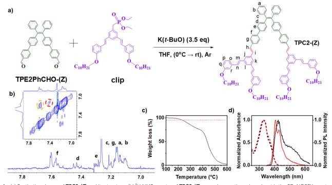
Fig. 1 (a) Synthetic scheme of TPC2-(Z) and its structure. (b) <sup>1</sup>H NMR spectra of TPC2-(Z) around aromatic regions. Inset is the 2D-NOESY spectrum of TPE2-(Z), (c) TGA result of TPC2-(Z) under nitrogen at 10 K min<sup>-1</sup> of heating rate. (d) UV-Vis absorption (dotted line) and the normalized PL spectra of  $10^{-5}$  M solution of **TPC2-(Z)** (black) and TPC2-(E + Z) in CHCl<sub>3</sub>
