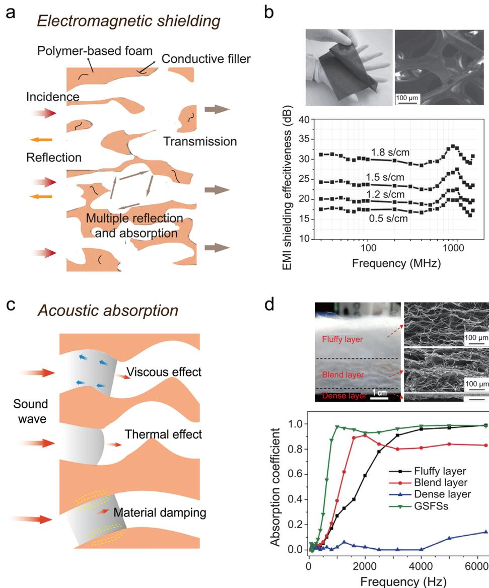
**Fig. 12** The porous polymers regulate electromagnetic and acoustic waves. (a) The mechanism of EMI shielding of porous materials. (b) The EMI shielding effectiveness of a graphene/PDMS composite foam. Reproduced with permission.<sup>41</sup> Copyright 2013, WILEY-VCH. (c) Schematic diagram of the energy consumption mechanisms of porous materials. (d) Gradient porous fibers serve as broadband sound absorption. Reproduced with permission.<sup>40</sup> Copyright 2021, Elsevier.
