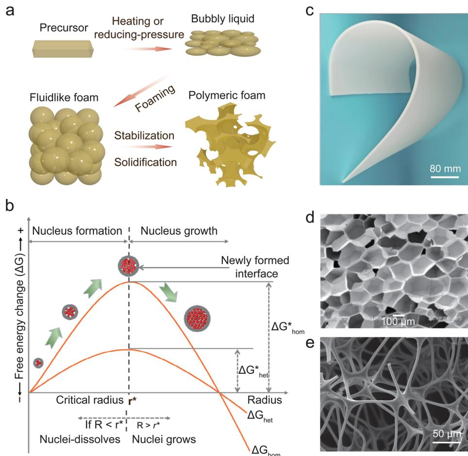
Fig. 6 Gas foaming to fabricate porous polymer foams. (a) Schematic of a typical blowing process. (b) Bubble nucleation and growth as a function of free energy. Reproduced with permission.<sup>114</sup> Copyright 2015, Elsevier. (c) Photo of commercial melamine foam fabricated by blowing technique. (d) and (e) Morphologies of a closed-pore structure (d) (reproduced with permission.<sup>118</sup> Copyright 2007, Elsevier) and an open-pore structure (e).
