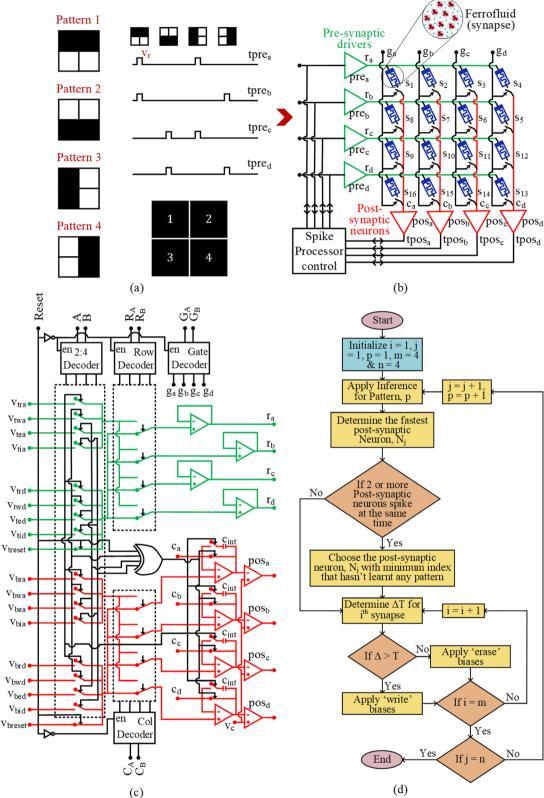
Fig. 9 (a) Numbering of the  $2 \times 2$  pixel and different patterns considered for learning, (b) scheme of the  $4 \times 4$  synaptic crossbar where the patterns are applied as read pulses across the rows, (c) scheme of the pre-synaptic drivers and post-synaptic neurons with their digital control signals, and (d) flowchart for carrying out spike-based unsupervised learning for pattern recognition.
