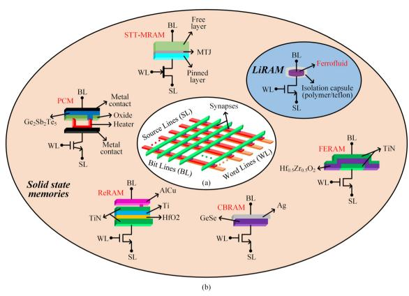
Fig. 1 (a) A fully connected memristive crossbar and (b) ferrofluid LiRAM (liquid random access memory) device structure compared with its solid state counterparts. 16-20
