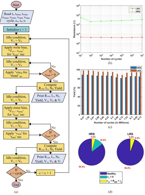
Fig. 7 (a) Flowchart for switching the EMG ferrofluid's resistance between HRS and LRS in pulse mode, (b) endurance test results of 10 million switching cycles between the LRS and HRS using a mean read voltage of 14 mV, (c) yield distribution of the HRS and LRS values for 10 million cycles using a mean read voltage of 14 mV, (d) factors affecting the yield of the HRS and LRS values.
