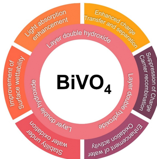
Fig. 4 Schematic illustration of the role of LDHs in enhancing the PEC performance of BiVO 4 photoanodes.
