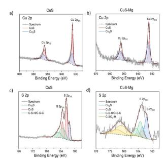
Fig. 3 XPS spectra of Cu 2p and S 2p for (a and c) CuS and (b and d) CuS-Ma
