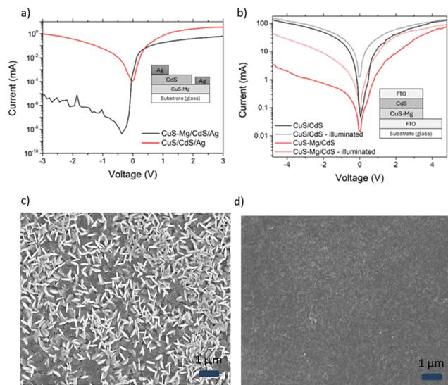
**Fig. 6** Current–voltage measurements for CuS/CdS and CuS–Mg/CdS with (a) Ag as the electrode and (b) FTO as the electrode. Schematics of the diode structures are included as insets. Dotted lines represent illumination conditions during the measurements. Plane-view SEM of (c) CuS and (d) CuS–Mg.
