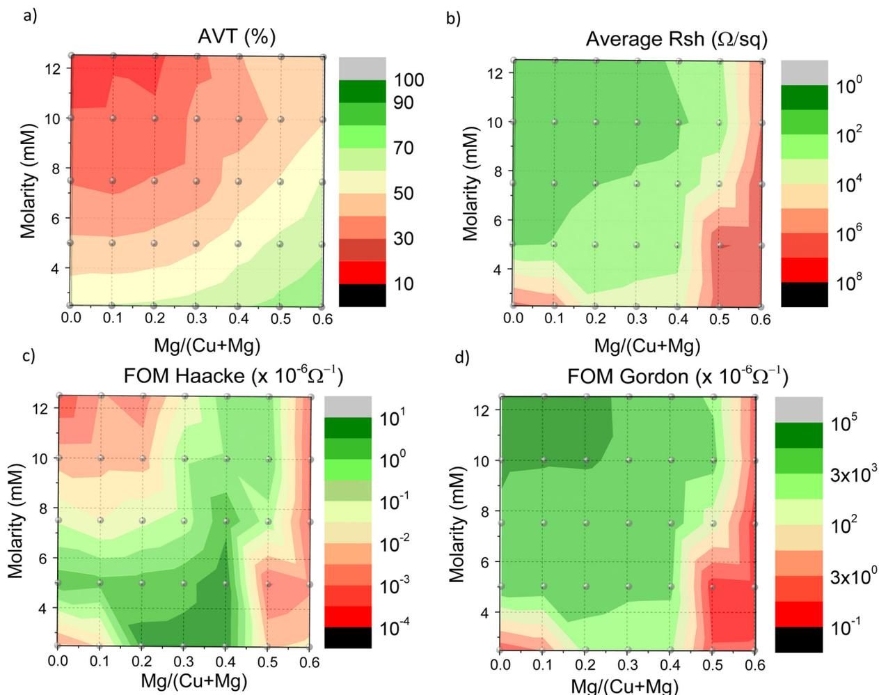
Fig. 1 Contour map of (a) average visible transmittance (AVT) (%), (b) average sheet resistance ( $R_s$ ) ( $\Omega \square^{-1}$ ), (c) FOM<sup>H</sup> ( $\times 10^{-6} \Omega^{-1}$ ) and (d) FOM<sup>G</sup> ( $\times 10^{-6} \Omega^{-1}$ ) with respect to Mg/(Mg + Cu) and molarity variation.
