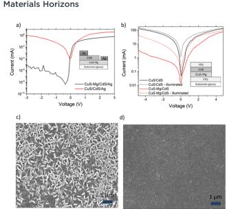
Fig. 6 Current-voltage measurements for CuS/CdS and CuS-Mg/CdS with (a) Ag as the electrode and (b) FTO as the electrode. Schematics of the diode structures are included as insets. Dotted lines represent illumination conditions during the measurements. Plane-view SEM of (c) CuS and (d) CuS-Mg.
