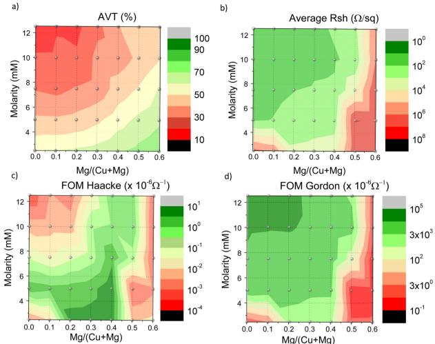
Fig. 1 Contour map of (a) average visible transmittance (AVT) (%), (b) average sheet resistance ( $R_s$ ) ( $\Omega$   $\Box^{-1}$ ), (c) FOM<sup>H</sup> ( $\times$  10<sup>-6</sup>  $\Omega^{-1}$ ) and (d) FOM<sup>G</sup> ( $\times$  10<sup>-6</sup>  $\Omega^{-1}$ ) with respect to Mg/(Mg + Cu) and molarity variation.
