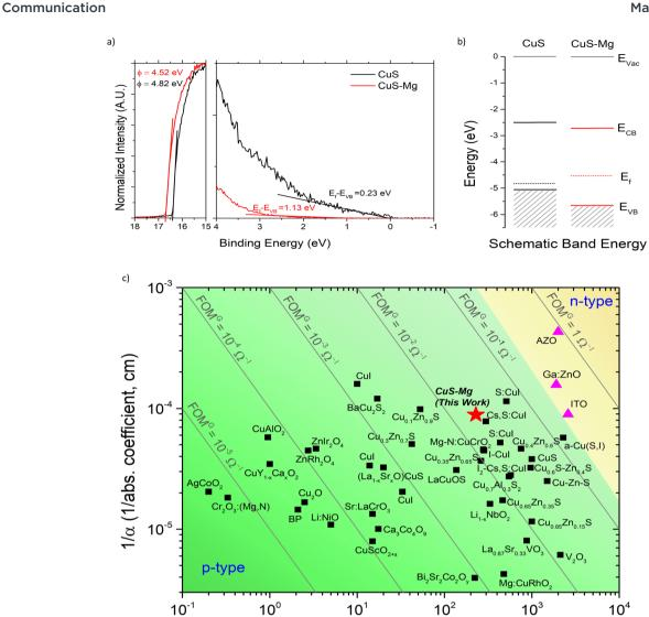
Fig. 5 (a) UPS spectra at the secondary electron cut off and valence band region. (b) Schematic band alignment of CuS and CuS-Mg. (c) List of different p-type transparent conducting materials as a function of inverse absorption coefficient at 550 nm and conductivity. The yellow area indicates the region of reported n-type transparent conducting oxides. The grey line indicates FOM<sup>G</sup> values.
