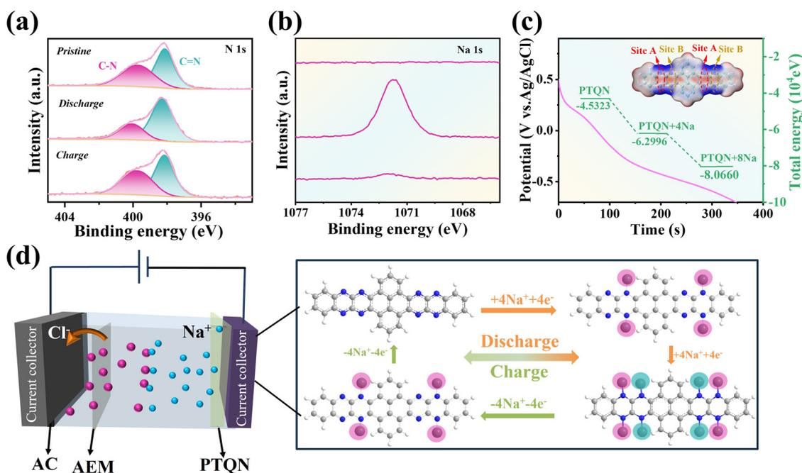
Fig. 4 *Ex situ* XPS spectra of (a) N 1s and (b) Na 1s collected at selected potentials, revealing the chemical states of nitrogen and sodium within the PTQN structure (c) Calculated total energies of sodium-intercalated PTQN structures, indicating stability variations with sodium incorporation. (d) Schematic diagram illustrating the mechanism of the PTQN electrode during the desalination process, depicting key electrochemical reactions and ion transport dynamics.
