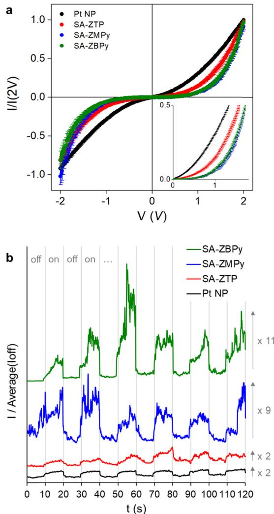
Fig. 5 Charge transport measurements at the nanoscale, performed by conductive AFM on **Pt NP**, **SA-ZTP**, **SA-ZMPy** and **SA-ZBPpy**, at room temperature. (a)  $I$ - $V$  curves; the curves are normalized at 2 V; inset: magnification of the 0–1 V region. (b) Evolution of the current intensity under light irradiation at a voltage of 2 V; light is successively switched on and off.
