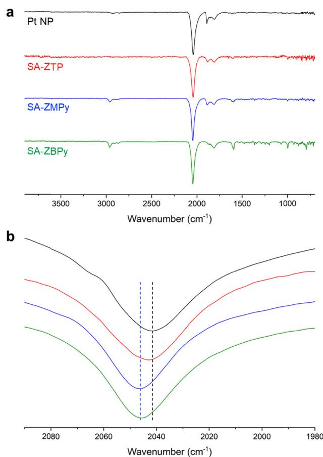
Fig. 3 Infrared spectra of the pristine **Pt NP** and of the **SA-ZTP**, **SA-ZMPy** and **SA-ZBPy** self-assemblies. (a) Full spectra and (b) zoomed-in view of the terminal CO region (the baselines are shifted for clarity – the dashed lines are a guide to the eye); peak maxima: **Pt NP**:  $2041 \text{ cm}^{-1}$ , **SA-ZTP**:  $2042 \text{ cm}^{-1}$ , **SA-ZMPy**:  $2046 \text{ cm}^{-1}$ , and **SA-ZBPy**:  $2046 \text{ cm}^{-1}$ .
