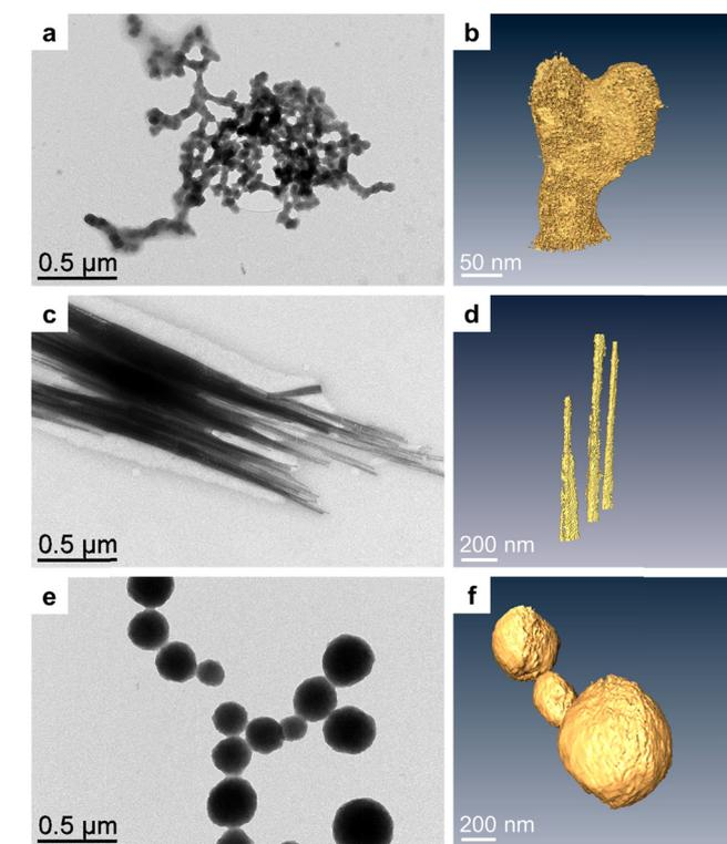
Fig. 2 TEM pictures of the self-assemblies of **Pt NP** with porphyrins. (a) and (b) **SA-ZTP**, (c) and (d) **SA-ZMPy** and (e) and (f) **SA-ZBPy** – (a), (c) and (e) low magnification images, and (b), (d) and (f) tomography 3D reconstruction.
