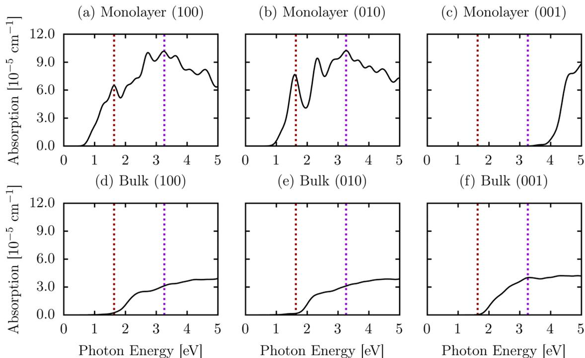
Fig. 5 Optical absorption activity of (a)–(c) monolayer goldene and (d)–(f) bulk-like goldene for incident light polarized along the  $x$ - (100),  $y$ - (010), and  $z$ -directions (001). The dashed red and violet lines mark the visible range of the optical spectrum.
