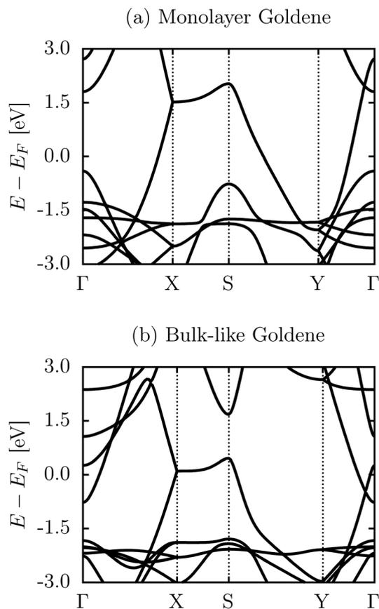
Fig. 3 The electronic band structure of (a) the goldene monolayer and (b) the bulk-like goldene model.
