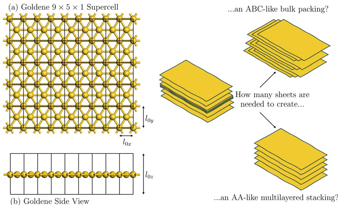
**Fig. 1** Schematic representation of goldene: front view (a) of a  $9 \times 5 \times 1$  supercell, highlighting the unit cell replications and the magnitudes of the lattice vectors  $l_{0x}$  and  $l_{0y}$ . Side view (b) of the goldene monolayer, indicating the lattice parameter in the out-of-plane direction  $l_{0z}$ . On the right, the main objective of this work: to determine how the stacking of goldene monolayers depends on the number of layers.
