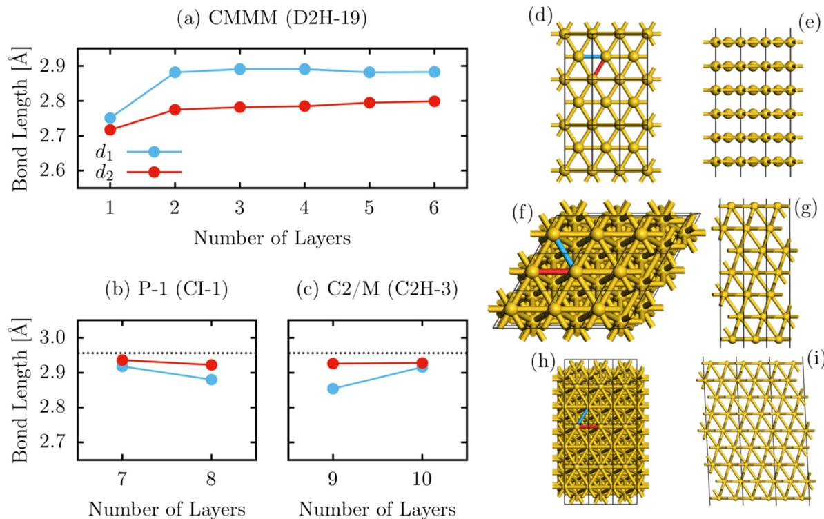
Fig. 7 (a) Evolution of two characteristic bond lengths, denoted as  $d_1$  (blue) and  $d_2$  (red), for goldene systems from one to six layers. Panels (b) and (c) show the bond lengths  $d_1$  and  $d_2$  for seven and eight layers and nine and ten, respectively. Panels (d)–(i) show the top and side views of representative cases for each group of the lattice arrangement presented in Fig. 6.
