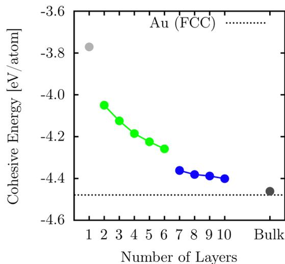
Fig. 6 Multilayered goldene's structural evolution as a layer number function, focusing on the cohesive energy. The dashed line refers to the cohesive energy for the FCC bulk gold.
