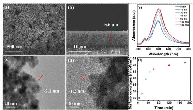
Fig. 2 SEM images of FTO|*nano*ITO from (a) (top view) and (b) cross-sectional view; (c) and (d) HRTEM images of *nano*ITO-RuCat|PI. (e) UV-vis absorption spectra of FTO|*nano*ITO electrodes after various soaking times in 150  $\mu\text{M}$  RuCat in methanol; (f) RuCat surface coverages after exposure for different times.
