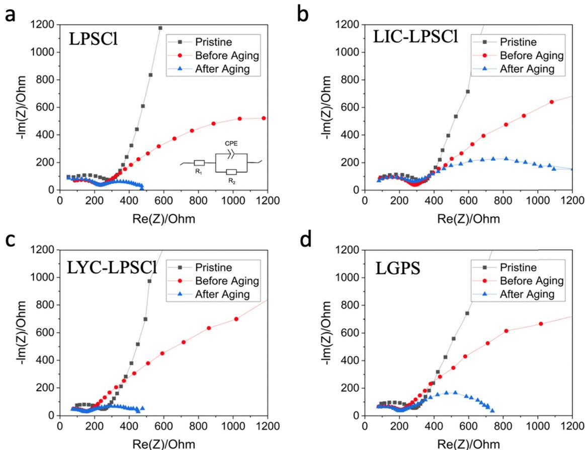
Fig. 3 EIS Nyquist plot for four different catholytes of (a) LPSCI, (b) LIC-LPSCI, (c) LYC-LPSCI, (d) LGPS. The inset of (a) includes the equivalent circuit model, with  $R_1$  representing bulk SSE resistance,  $R_2$  representing interfacial resistance, and CPE presenting the constant phase element.
