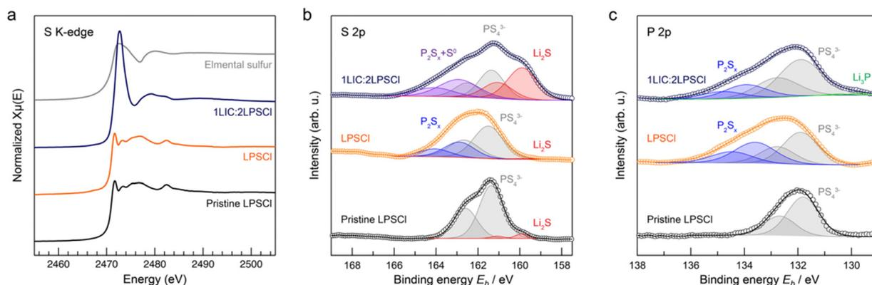
**Fig. 6** (a) Normalized XANES spectra at the S K-edge for pristine LPSCI–NMC811, aged NMC811 with LPSCI and LIC–LPSCI catholytes, and elemental sulfur as a control. (note that S XAS data were collected from the cycled cell); XPS spectra of (b) the S 2p, and (c) the P 2p orbitals for pristine LPSCI, aged LPSCI catholyte and LIC–LPSCI catholyte, illustrating the decomposition pathway of LIC–LPSCI.
