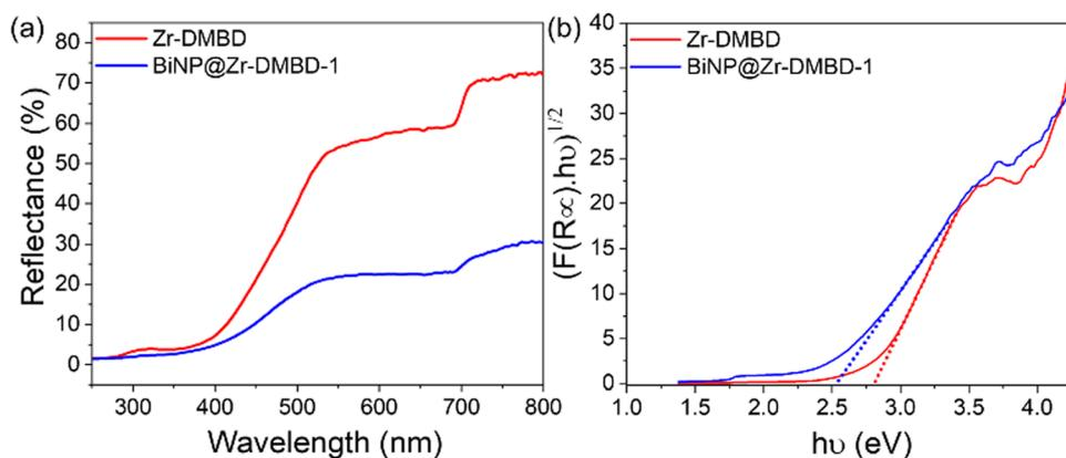
Fig. 8 (a) UV-Vis DRS of Zr-DMBD (red line) and  $\text{BiNP@Zr-DMBD-1}$  (blue line). (b) Tauc plot of Kubelka–Munk function for bandgap determination of Zr-DMBD (red line) and  $\text{BiNP@Zr-DMBD-1}$  (blue line).
