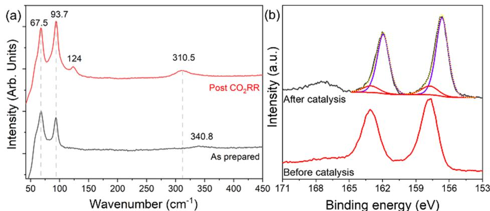
**Fig. 7** Comparison of as-prepared and post CO<sub>2</sub>RR characterization of BiNP-Zr-DMBD-1 (a) Raman spectra and (b) high resolution Bi 4f XPS. Broad peak around 168 eV on Post CO<sub>2</sub>RR XPS spectra (black line) can be attributed to S 2s originating from the Nafion binder.
