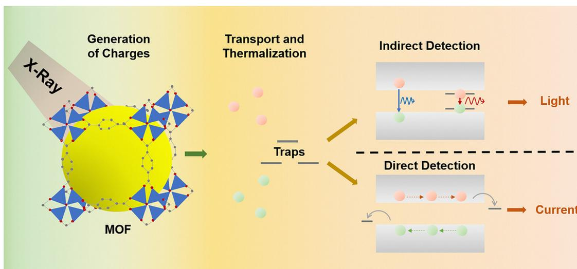
**Fig. 1** Free charges are generated by the interaction of the X-ray with the MOF. For indirect detection (scintillation), the incident X-rays are down-converted to photons which are collected by a photodetector. For direct detection, the incident X-rays are directly converted into current which are collected at the electrodes.
