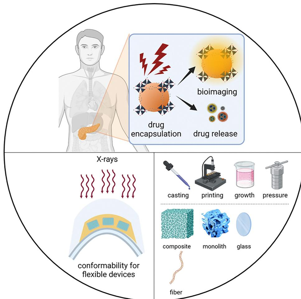
**Fig. 6** Some applications and opportunities for MOF-based X-ray detectors and scintillators, and production methods. (Top) Targeted drug delivery and bioimaging using MOFs in the human body. (Bottom left) Conformability of MOFs into flexible films and devices. (Bottom right) Some fabrication methods of various MOF morphological assemblies towards scalable production. The monolith illustration was adapted with permission from ref. 29 and 91. Created with BioRender.com.
