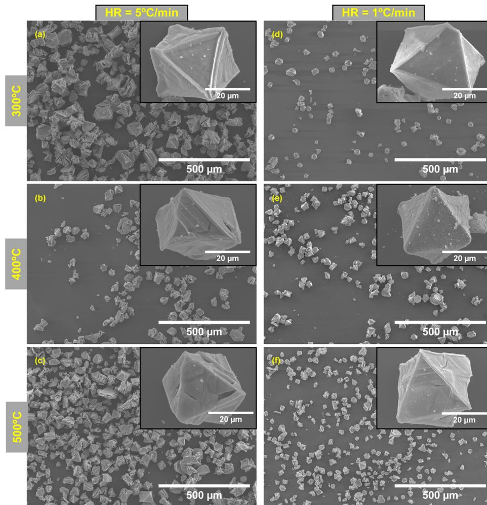
Fig. 4 SEM of the synthesized P-CuO<sub>x</sub> at 300 °C (a) and (d), 400 °C (b) and (e), and 500 °C (c) and (f), for 1 h duration, With HR of 5 °C min<sup>-1</sup> (left column) and 1 °C min<sup>-1</sup> (right column).
