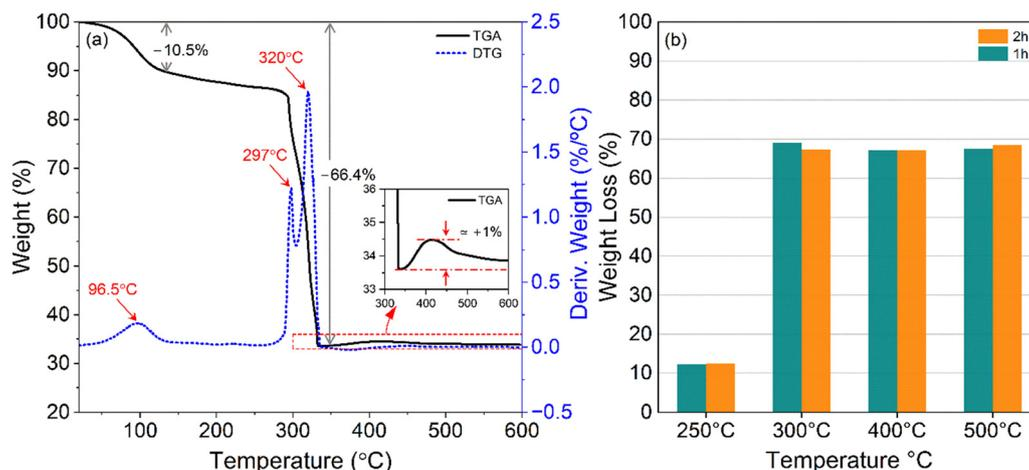
Fig. 3 (a) TGA and DTG of Cu-BTC in air. (b) Calculated weight loss of heat-treated Cu-BTC.
