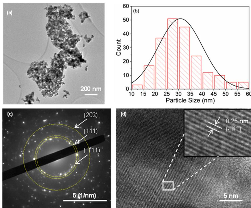
Fig. 5 (a) TEM image of the synthesized P-CuO at  $500\text{ }^{\circ}\text{C}$  (with HR of  $5\text{ }^{\circ}\text{C min}^{-1}$  for 1 h); and the respective (b) particle size histogram distribution, (c) selected area electron diffraction (SAED) pattern, and (d) lattice-resolved image collected from the region enclosed in a white rectangle.
