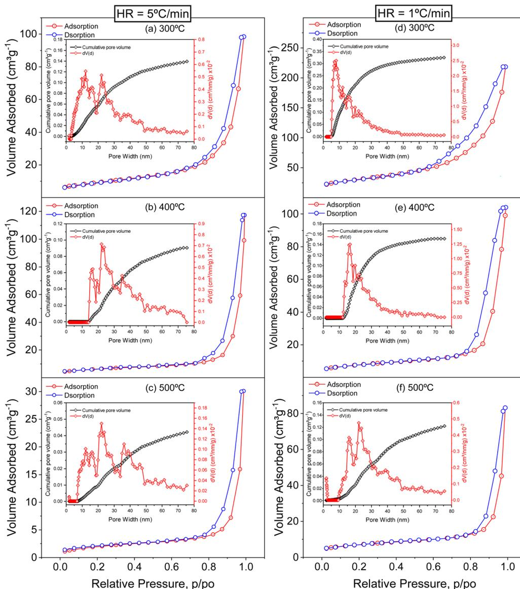
Fig. 9  $N_2$  Adsorption–desorption isotherms, with insets presenting the corresponding pore size distribution, for the synthesized P-CuO<sub>x</sub> at different  $T_C$ : (a) and (d) 300 °C, (b) and (e) 400 °C, and (c) and (f) 500 °C, for 1 h duration, with different HR, 5 °C min<sup>-1</sup> (left column) and 1 °C min<sup>-1</sup> (right column).
