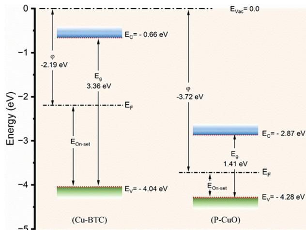
Fig. 8 Energy level band diagram of pristine Cu-BT (left side) and the synthesised P-CuO sample (right side,  $T_C$  of 500 °C, HR of 5 °C min<sup>-1</sup> for 1 h).
