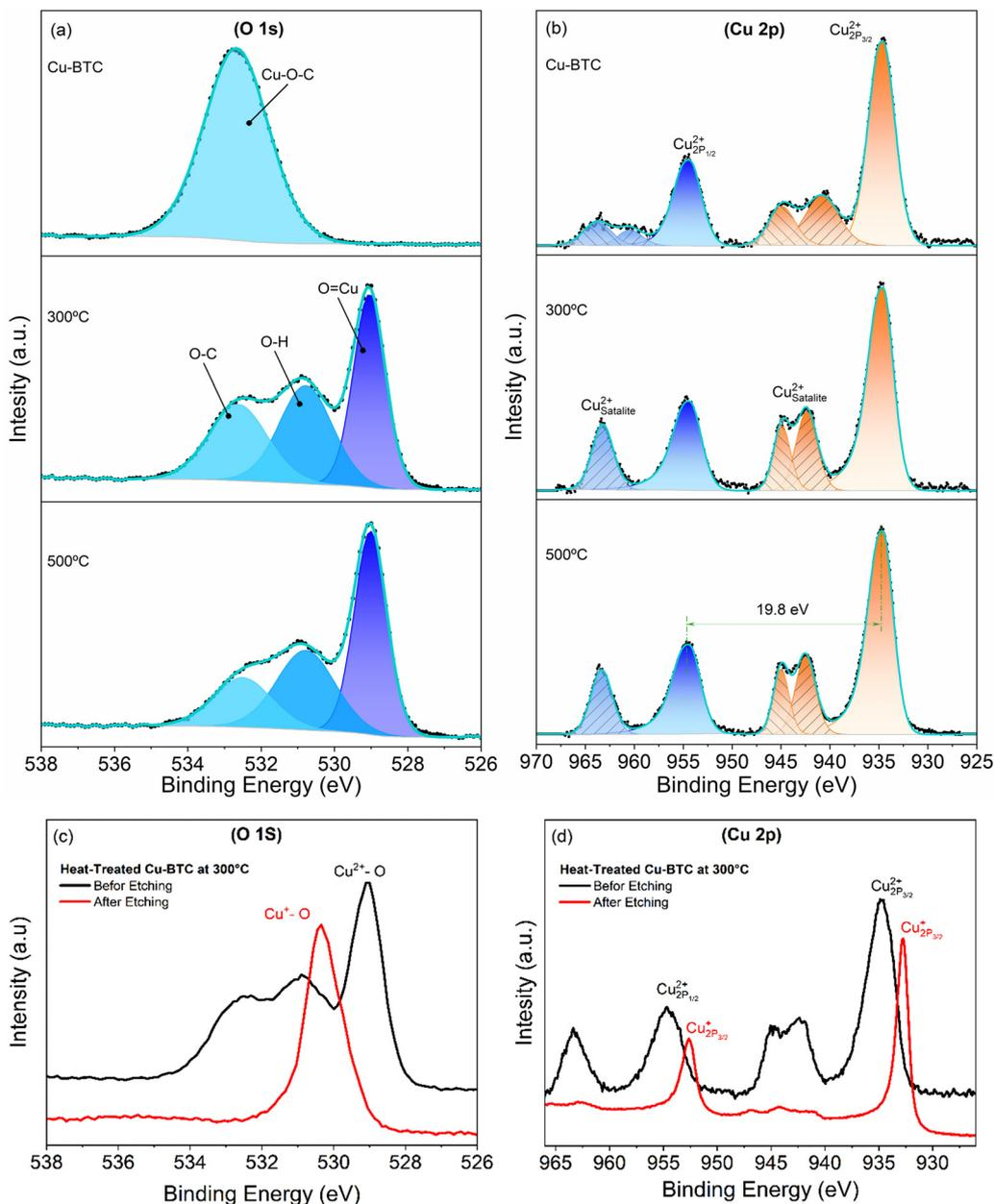
Fig. 6 (a) and (b) High resolution spectrum of O 1s (a) and Cu 2p (b) XPS spectra of pristine Cu-BTC and the synthesized P-CuO<sub>x</sub> at 300 and 500 °C (with HR of 5 °C min<sup>-1</sup> for 1 h). (c) and (d) O 1s and Cu 2p spectra, respectively, for the sample treated at 300 °C after applying ion-beam based surface etching.
