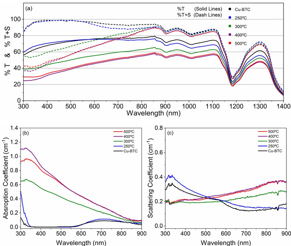
Fig. 10 (a) Transmittance (%  $T$ ) and transmittance plus scattering (%  $T + S$ ) of pristine Cu-BTC and the synthesized P-CuO<sub>x</sub> at different  $T_C$  (HR of 5 °C min<sup>-1</sup> for 1 h), and the corresponding (b) absorption and (c) scattering coefficients.
