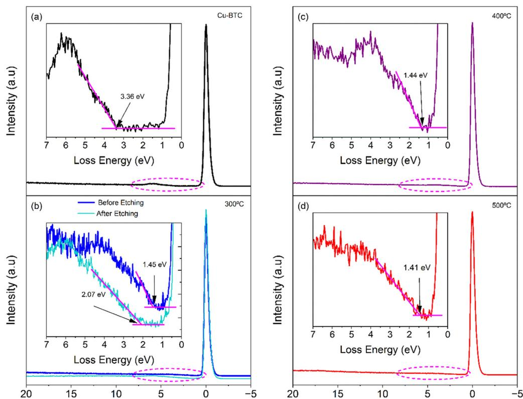
Fig. 7 REELS spectra of (a) pristine  $\text{Cu-BTC}$  and the  $\text{P-CuO}_x$  synthesized at (b) 300 °C (before and after surface etching), (c) 400 °C, and (d) 500 °C. Insets display the low-energy loss region, highlighting the band gap transition.
