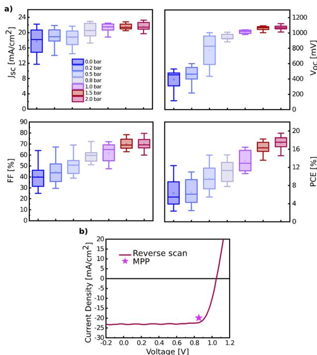
**Fig. 8** (a) Statistical photovoltaic parameters of short-circuit photocurrent density ( $J_{sc}$ ), open-circuit voltage ( $V_{oc}$ ), fill factor (FF), and power conversion efficiency (PCE). (b)  $J-V$  curves of a champion solar cell prepared with evaporation rate of 2 bar.
