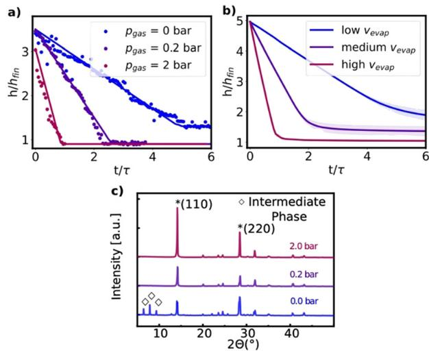
**Fig. 3** Drying film height in experiment (a) and in simulation (b). The lines in the experimental data are added as a guide for the eye.  $\tau$  is the time until the film has reached its dry film height for the fastest evaporation rate. For the simulation, the shaded area indicates one standard deviation from the mean value. (c) XRD after drying.
