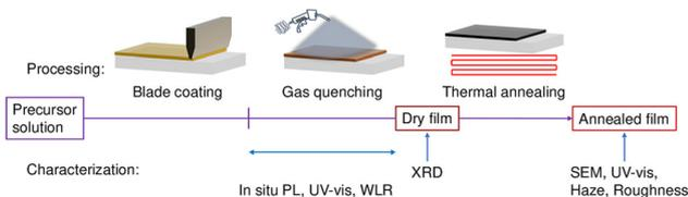
**Fig. 2** Schematic diagram of the experimental fabrication and characterization process. The precursor solution is blade-coated onto the substrate followed by gas quenching treatment at different air pressures. During gas quenching either a PL or a WLR signal is recorded. The XRD spectra are taken on the dry film before annealing. Further measurements are performed after annealing.
