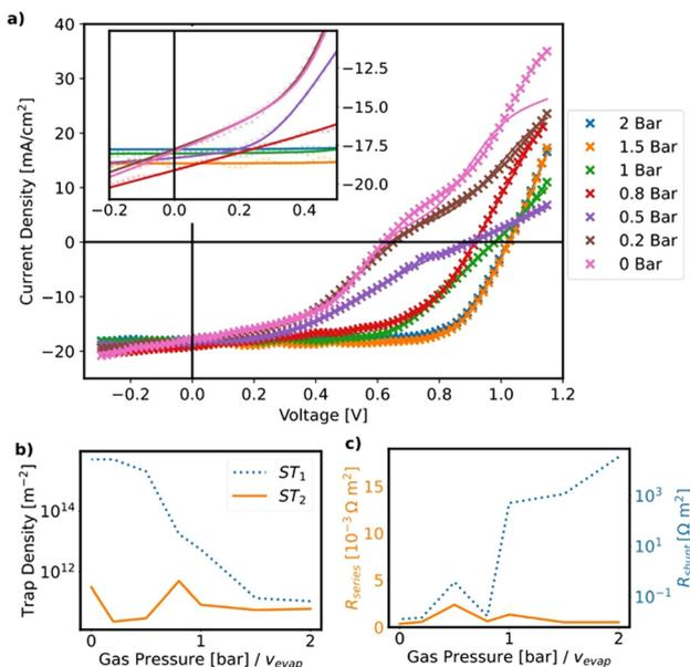
**Fig. 9** (a)  $JV$  curves fitted with a drift-diffusion model (experimental: crosses, fit: solid lines) and zoom around  $J_{sc}$  (inset). (b) and (c) Fitted parameters of the drift-diffusion model. (b)  $ST_1$  and  $ST_2$  are the interfacial trap densities between  $\text{SnO}_2$  and the perovskite, P3HT and the perovskite respectively, (c)  $R_{series}$  and  $R_{shunt}$  are the series and shunt resistances.
