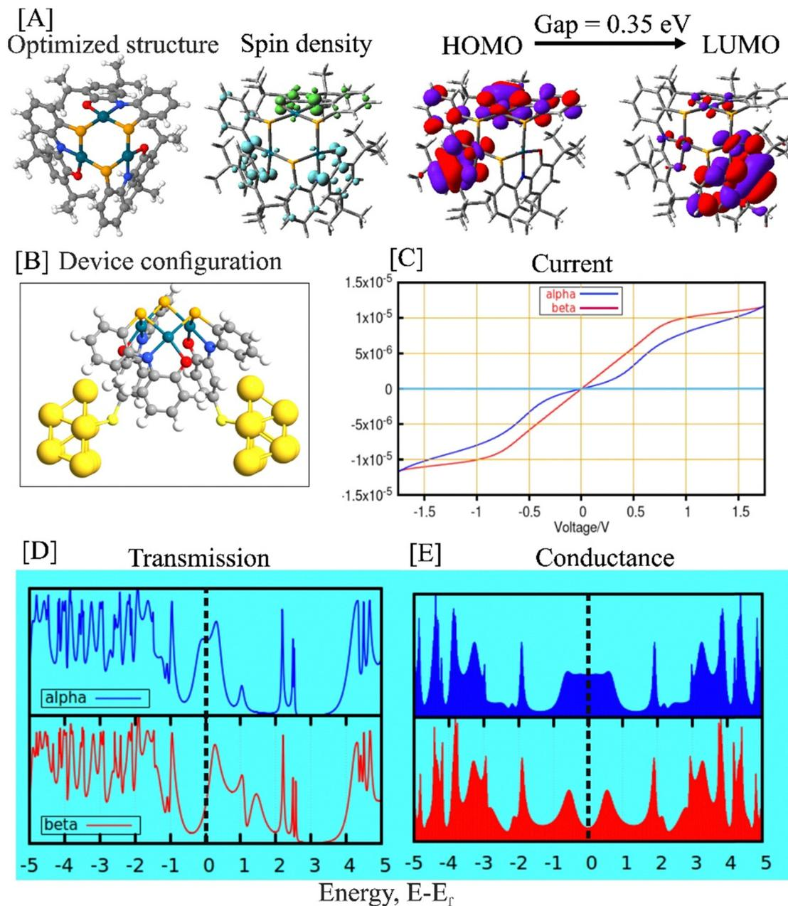
Fig. 2 (A) The DFT optimized structure of the neutral complex (complex **1**) along with the spin-density and FMOs at  $\omega$ B97XD/cc-pVDZ level. (B) Device configuration for the computed transmission characteristics of complex **1** with gold electrodes. The relative variations in: (C) current; (D) electronic transmission; and (E) conductance. The different color plots represent computed parameters for different electronic spins.
