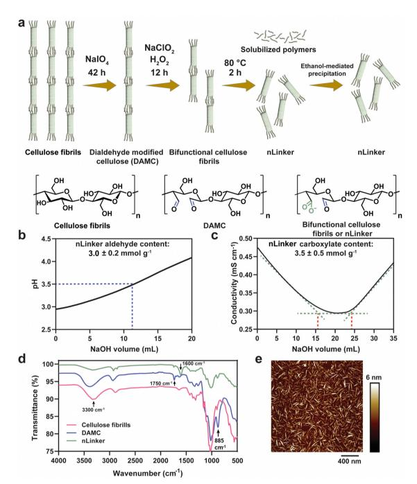
Fig. 2 nLinker synthesis and characterization. (a) Schematic of nLinker synthesis via successive periodate-chlorite oxidation reactions, as well as the corresponding changes in cellulose chemical structure. (b) A representative aldehyde titration curve of nLinker. (c) A representative carboxylate titration curve of nLinker using a strong base (10 mM NaOH). (d) ATR-FTIR spectra of cellulose fibrils, DAMC, and nLinker. (e) An AFM image of the nLinker.
