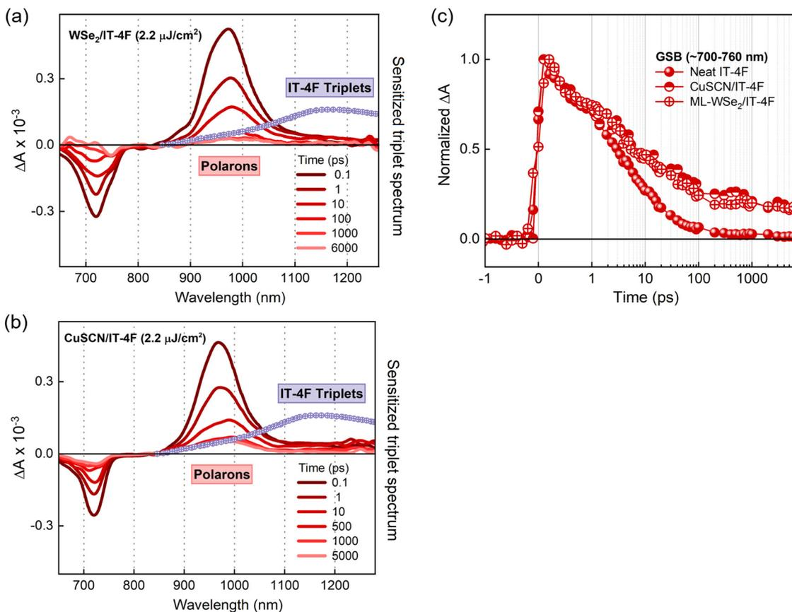
Fig. 4 Fluorination suppresses triplet generation. Series of transient absorption spectra of (a) ML-WSe<sub>2</sub>/IT-4F and (b) CuSCN/IT-4F bilayers (both excited at 700 nm and at a pump fluence of 2.2 μJ cm<sup>-2</sup>) with the sensitized triplet spectrum of IT-4F overlaid, and (c) the corresponding transient kinetics probed at the ground state bleach (GSB) signals.
