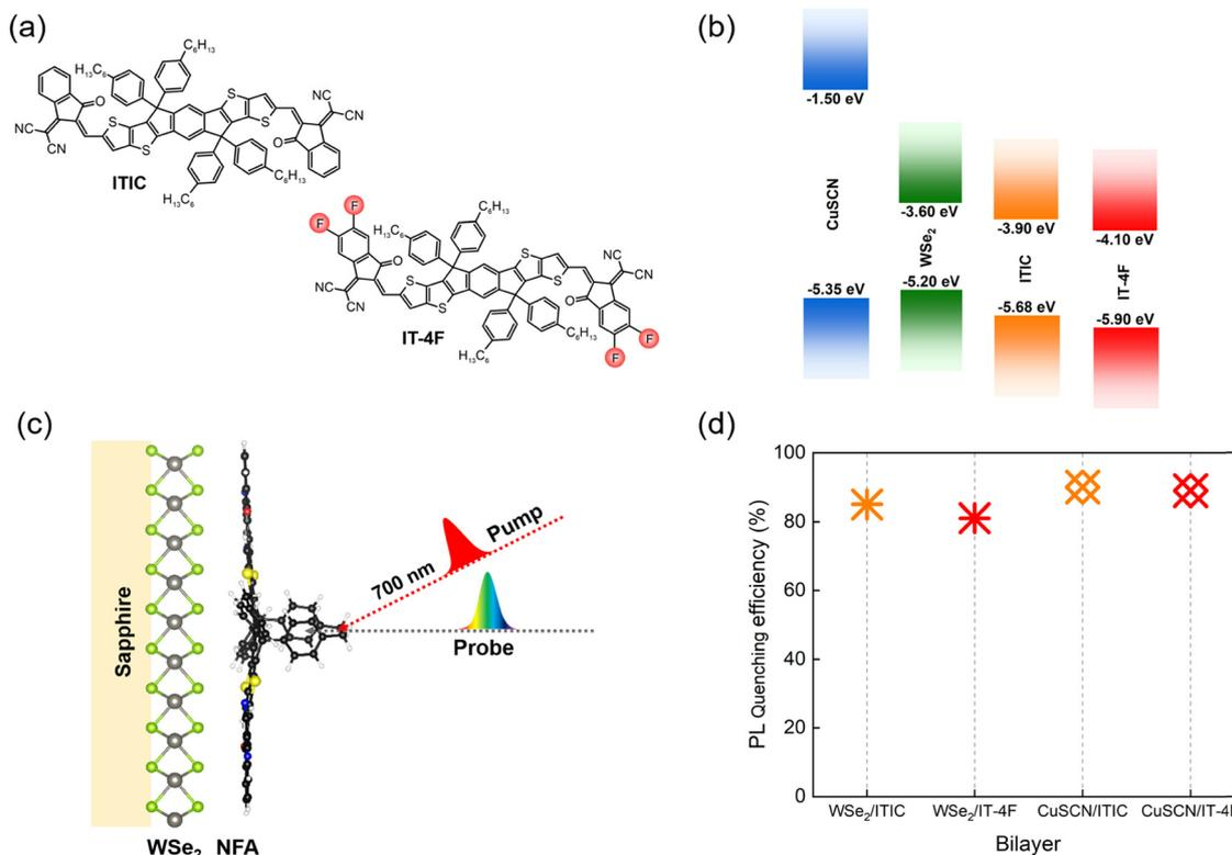
**Fig. 1** Active layer components and photoluminescence quenching. (a) Molecular structures of the NFAs, ITIC and IT-4F; (b) energy band diagram of donor materials (ML-WSe<sub>2</sub> and CuSCN) and NFAs where all the energy values are taken from the literature;<sup>25–27</sup> (c) schematic structure of the active layer; (d) photoluminescence quenching efficiencies in ML-WSe<sub>2</sub>/NFA and CuSCN/NFA bilayers (the corresponding PL spectra are given in Fig. S2, ESI†).
