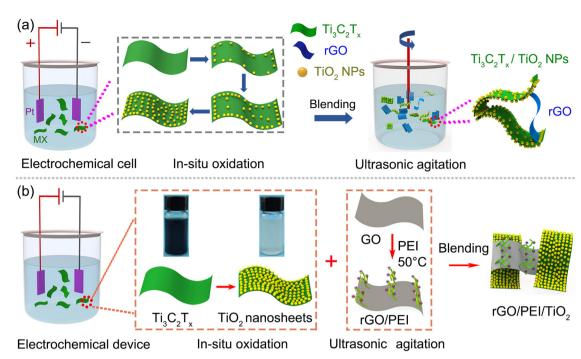
Fig. 8 Solution blending method for preparing graphene-based hybrids as (a)  $T_{13}C_2T_x/T_{10}$  NPs/rGO. Reproduced with permission. <sup>105</sup> Copyright from 2024, Wiley-VCH. (b) rGO/PEI/TiO<sub>2</sub>. Reproduced with permission.<sup>106</sup> Copyright from 2023, Elsevier.
