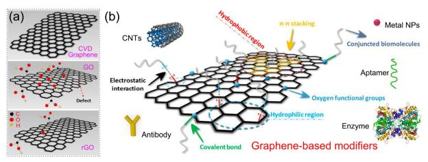
Fig. 7 Surface functionalization/decoration of graphene: (a) graphene and its derivatives. (b) Schematic of various modifiers functionalized on graphene. Reproduced with permission. 100 Copyright from 2019, Multidisciplinary Digital Publishing Institute.
