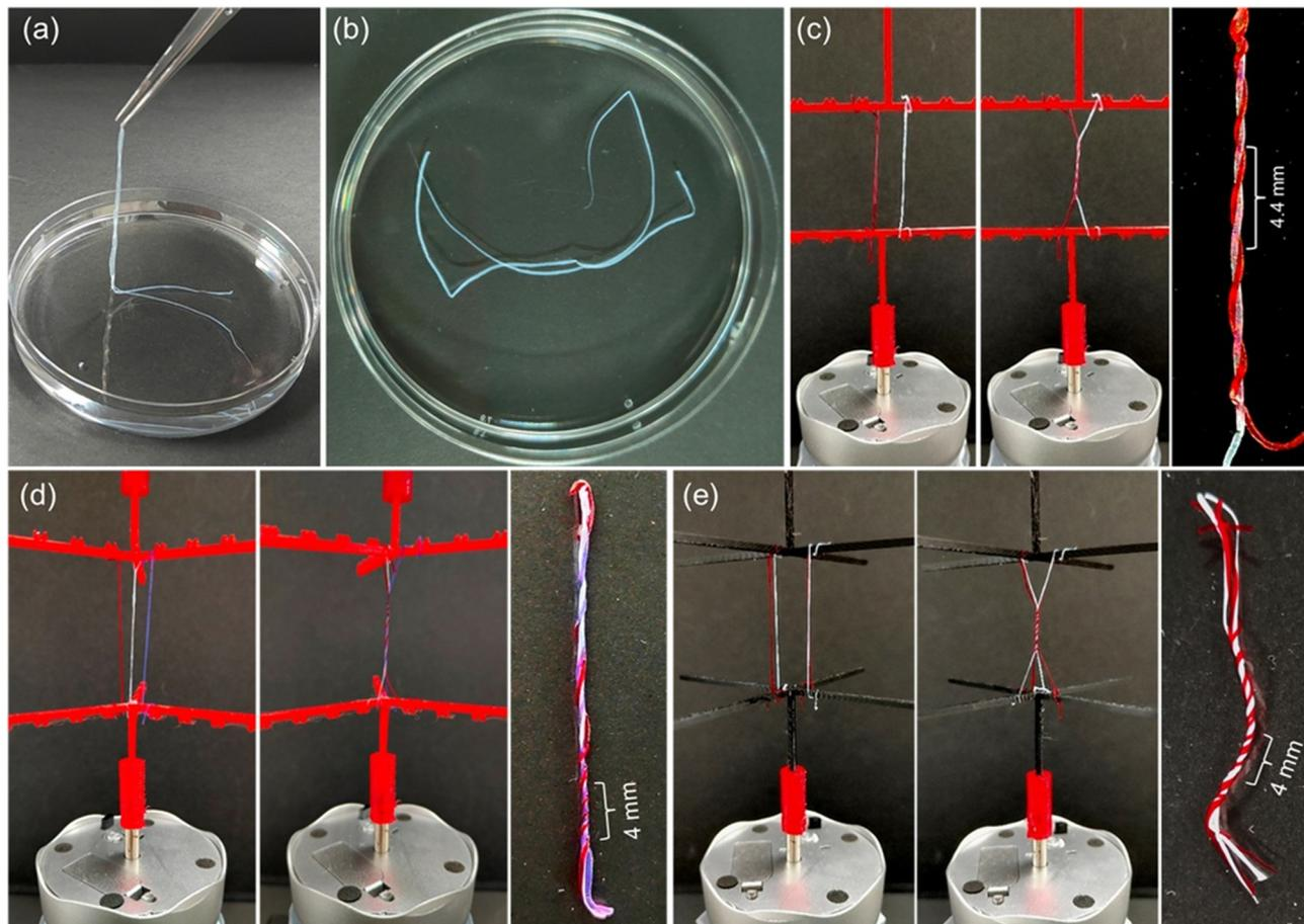
**Fig. 2** (a) Joining two 2NapFF noodles side-by-side, (b) separation of the noodles in water. (c–e) Twisting two, three, and four 2NapFF noodles using a rotating motor (at bottom end): before twisting (left), after 5 twists (middle), and the resulting twisted noodle (right). The red and blue noodles are stained with Congo red and bromocresol green for distinction. The grip-to-grip distance is 40.5 mm before twisting and 40 mm after twisting.
