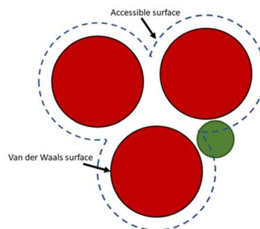
**Fig. 2** Illustration of solvent-accessible surface area (SASA) estimation using 1.4 Å probe radius, green sphere (FreeSASA) rolled over the MIP atoms, red spheres. Blue mesh regions denote regions accessible to solvent prior to crosslinking.
