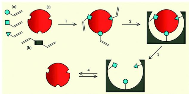
**Fig. 1** Generalised schematic of the molecular imprinting process involving (a) functional monomers, (b) crosslinker and (c) template. The workflow illustrates (1) template–monomer complexation in solution, (2) polymerisation in the presence of porogen, (3) extraction of template and solvent to yield a porous MIP structure with accessible recognition sites and (4) rebinding.
