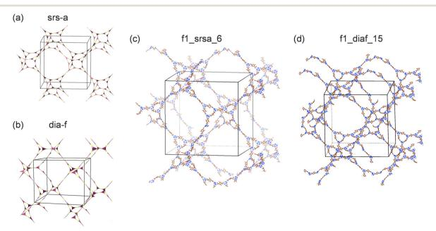
Fig. 7 Example structures with "vacant" topologies, (a) srs-a and (b) dia-f. The corresponding MOF structures (c) and (d) reach 1017 mg g<sup>-1</sup> and 1018 mg g<sup>-1</sup> gravimetric deliverable capacity, respectively.
