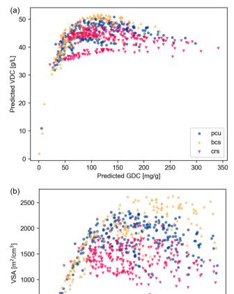
Fig. 11 Analysis of MOFs with pcu net and its polymorph nets, bcs and crs. Scatter plots displaying (a) predicted VDC against predicted GDC and (b) VSA against GSA. Data points are represented with blue circles for pcu-MOFs, orange upward triangles for bcs-MOFs (with higher net density than pcu), and red downward triangles for crs-MOFs (with lower net density than pcu)
