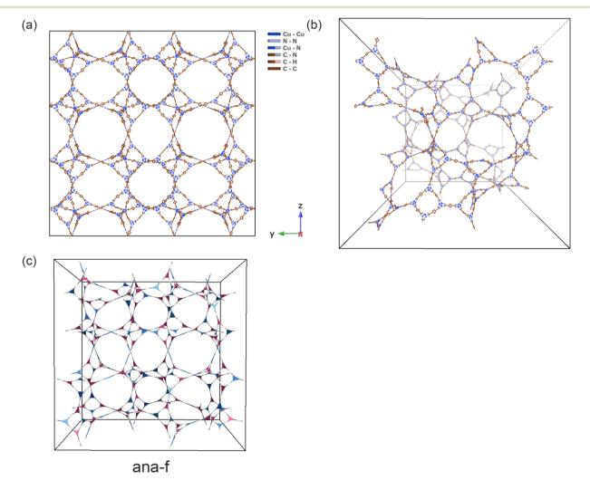
Fig. 3 The crystal structure of MOF f5\_anaf\_21: (a) parallel view, (b) perspective view, (c) perspective view of the ana-f net. Its unit cell volume of 9141330 Å<sup>3</sup> renders it extremely costly for GCMC simulations.
