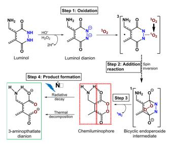
Scheme 2 Chemiluminescence of luminol in aprotic solvents, starting with the oxidation to luminol dianion (step 1), followed by addition reaction and spin inversion of molecular oxygen (step 2). Upon nitrogen elimination and formation of chemiluminophore (step 3), 3-aminophthalate is formed via chemiexcitation, followed by radiative or non-radiative decay (step 4).
