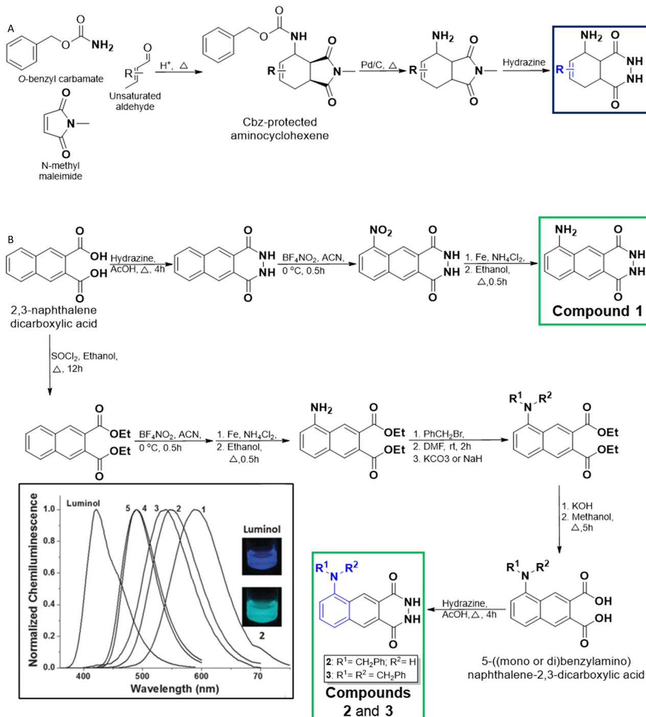
**Fig. 2** (A) Schematic representation of the synthesis of alkyl luminol derivatives. (B) Synthetic routes of luminol derivatives with naphthalene, and the corresponding CL emission spectra in H<sub>2</sub>O/DMSO solution with potassium persulfate in the inset. Reprinted with permission.<sup>49</sup>
