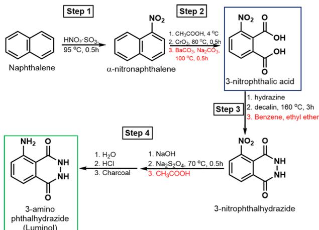
**Scheme 1** Luminol synthesis pathways, starting with naphthalene nitration (step 1), followed by oxidation to 3-nitro-phthalic acid (step 2), which, upon hydrazinolysis (step 3), and subsequent treatment with NaOH, sodium dithionite, and acidic precipitation yield luminol (step 4).
