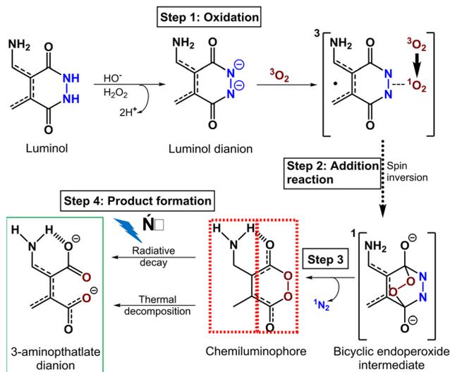
**Scheme 2** Chemiluminescence of luminol in aprotic solvents, starting with the oxidation to luminol dianion (step 1), followed by addition reaction and spin inversion of molecular oxygen (step 2). Upon nitrogen elimination and formation of chemiluminophore (step 3), 3-aminophthalate is formed *via* chemiexcitation, followed by radiative or non-radiative decay (step 4).
