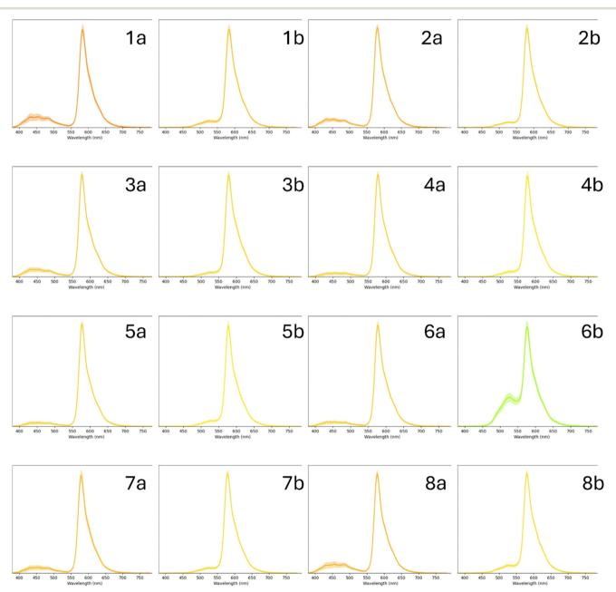
Fig. 3 Emission spectra of all OLEDs with fluorescent emitters 1-8 taken at L = 250 cd m<sup>-2</sup>. All spectra marked as (a) are devices without TxO-PhCz and those marked with (b) have 20% nominal TxO-PhCz. The blurring of the spectra denotes the standard deviation of the spectra due to compositional variation.
