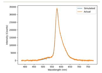
Fig. 7 Sample spectral output for the FD = BuO-BsubPc (4) hyperfluorescent OLEDs, showing the measured emission and the deconvoluted emission; ~525 nm being the emission of the TADF assistant and the ~575 nm being the BuO-BsubPc emission (as an example)
