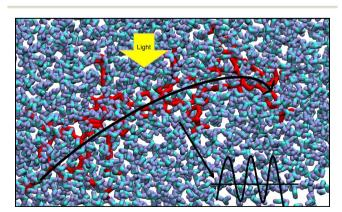
Fig. 1 A graphical representation of the TPPS<sub>4</sub> tetramer light absorption and optical spectra generation. The photosensitizer (TPPS<sub>4</sub> tetramer) is irradiated with light and the resulting optical spectra, which can be measured with a spectrometer, are shown.
