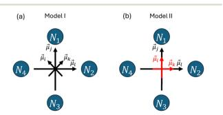
Fig. 6 Models (a)-I and (b)-II of optical transition dipole orientations in relation with the TPPS<sub>4</sub> molecule's nitrogen atoms, with  $\vec{\mu}_i$  and  $\vec{\mu}_k$  corresponding to the optical transition energies of the Q band and  $\vec{\mu}_j$  and  $\vec{\mu}_l$  for the B band.
