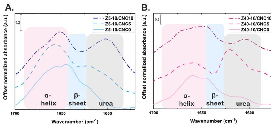
Fig. 5 PTIR investigation of the amide I region ( $1700$ – $1600$   $\text{cm}^{-1}$ ) of A. Z5-10/CNC series and B. Z40-10/CNC series as a function of CNC weight fraction.
