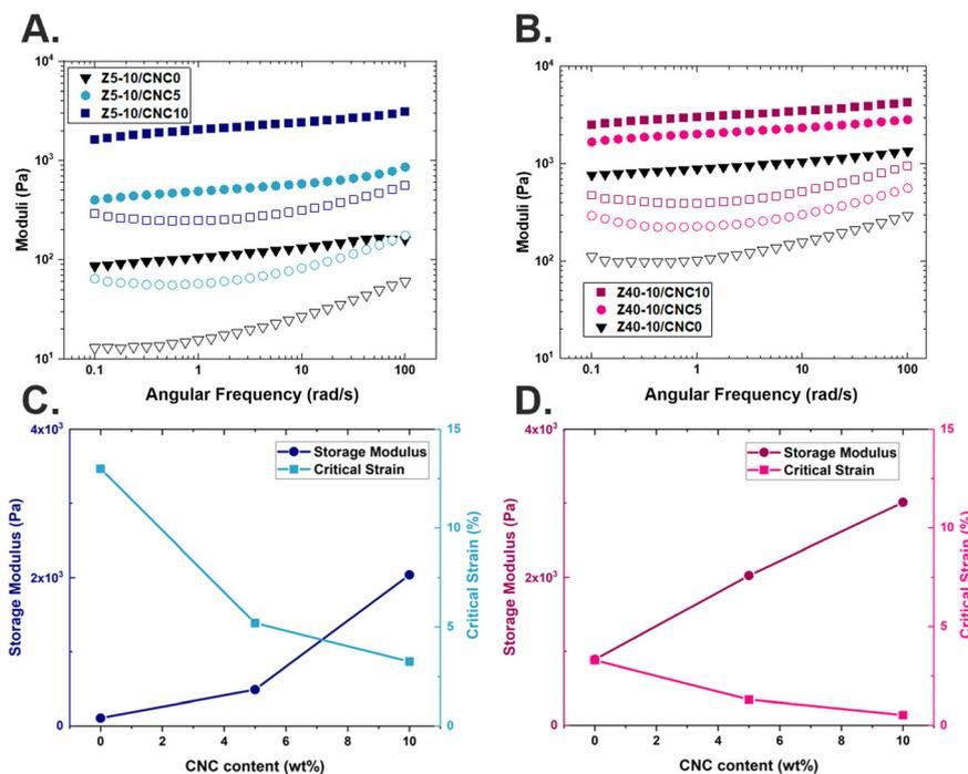
**Fig. 3** A) Angular frequency sweeps of Z5-10/CNC series and B) Z40-10/CNC series at 37 °C; open symbols indicate the storage moduli ( $G'$ ), and closed symbols indicate the loss moduli ( $G''$ ). Summary of trends in  $G'$  at 1 rad  $s^{-1}$  and critical strain as a function of CNC loading for C) Z5-10/CNC series and D) Z40-10/CNC series.
