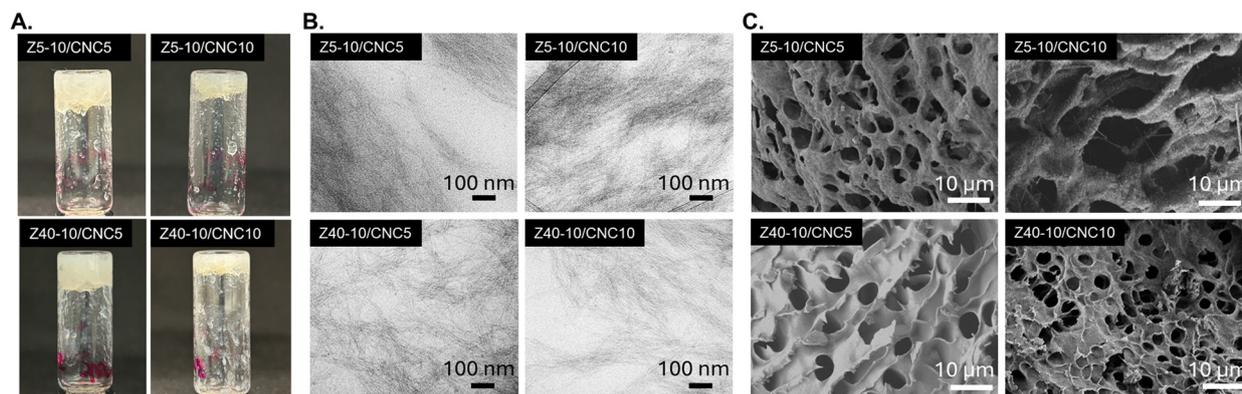
**Fig. 2** A. Vial inversion experiments of PPU/CNC nanocomposite hydrogels confirming gelation at 5 and 10 wt% CNC loading. B. Cryo-TEM images of Z5-10/CNC5, Z5-10/CNC10, Z40-10/CNC5, and Z40-10/CNC10 reveal fibrous structures in all PPU/CNC nanocomposites. C. SEM images of Z5-10/CNC0, Z5-10/CNC10, Z40-10/CNC5, and Z40-10/CNC10 show continuous porous networks.
