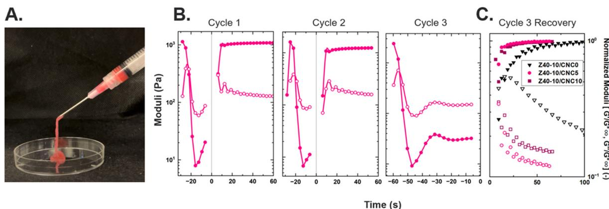
**Fig. 6** A. Injection demonstration of Z40-10/CNC5 hydrogel through an 18-gauge needle; a small amount of red food dye was added to the hydrogel as a visual aid. B. Step-strain recovery cycles for Z40-10/CNC5. C. Third recovery cycle of Z40-10/CNC0, Z40-10/CNC5 and Z40-10/CNC10. Open symbols indicate the loss moduli, while closed symbols indicate storage moduli.
