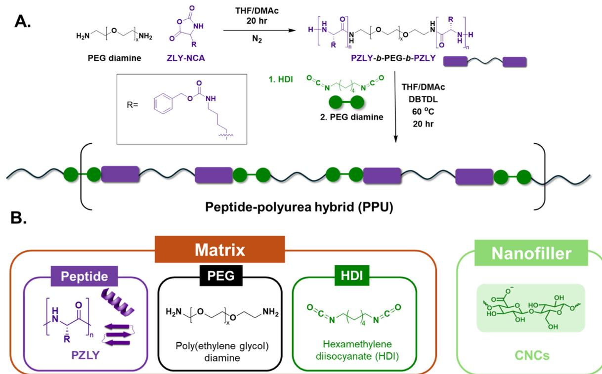
Fig. 1 A. Synthetic scheme of PPU hydrogel matrix. B. Components (matrix and nanofiller) of PPU/cellulose nanocrystal (PPU/CNC) nanocomposite hydrogels.
