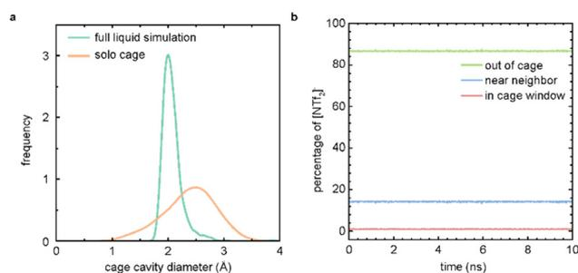
**Fig. 4** (a) Cage cavity diameter distribution over the course of the full liquid simulation (teal) and a simulation featuring one cage molecule simulated in gas (orange); (b) percentage of the NTf<sub>2</sub> counterions in cage windows (red), near neighbour (blue), and in the bulk solvent (green) over the course of the 10 ns simulation.
