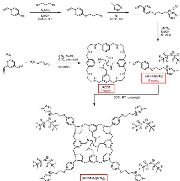
**Fig. 1** Synthesis of ionic liquid functionalised aldehyde  $[\text{Ald-IM}][\text{NTf}_2]$ , reduced organic cage **RCC1**, and formation of an ionic liquid-functionalised cage  $[\text{RCC1-IM}][\text{NTf}_2]_6$  –  $[\text{RCC1-IM}][\text{NTf}_2]_6$  includes six aminated-tied ionic liquid functional groups but only four are shown for clarity, with the remaining two linking together the connected diamines *via* the dashed lines.
