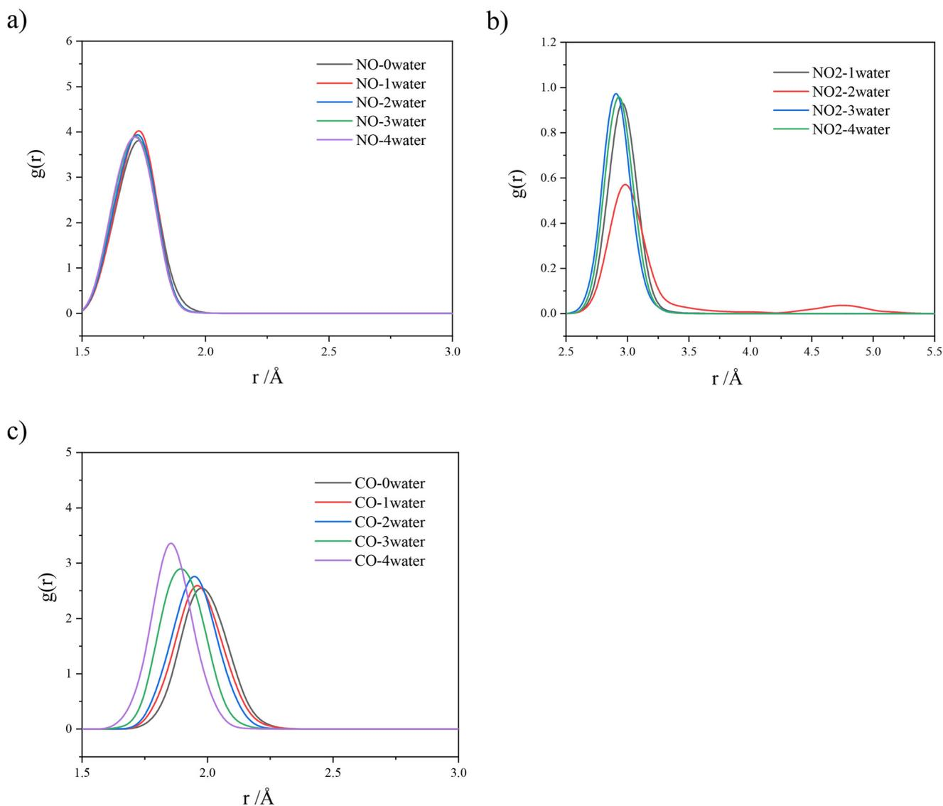
Fig. 5 RDFs between site-II Fe and (a) NO, (b)  $\text{NO}_2$ , and (c) CO respectively, in the presence of  $n = 0, 1, 2, 3$  and  $4 \text{ H}_2\text{O}$  molecules. Isolated  $\text{NO}_2$  RDF is omitted as it escapes site-II Fe.
