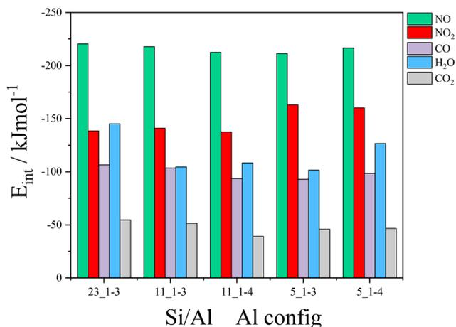
Fig. 3 Interaction energies computed at the PBE + D2 + U level of theory of NO, NO<sub>2</sub>, CO, H<sub>2</sub>O and CO<sub>2</sub> on Fe-MOR. The adsorption sites considered are characterized by Si/Al = {23, 11, 5}, 6MR topology, and Al distributions 1–3 and 1–4.
