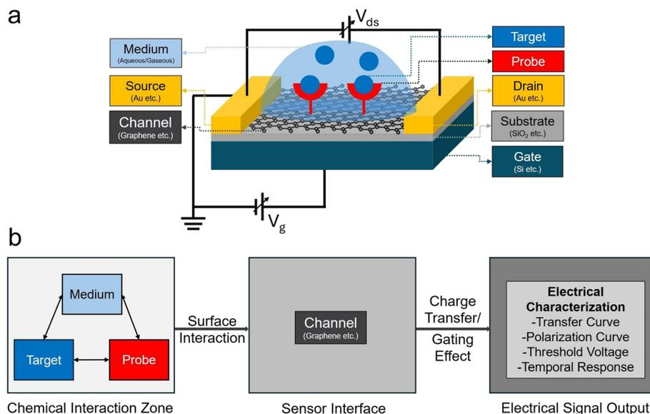
**Fig. 1** (a) Schematic illustration of a typical FET chemical sensor showing key structural components. (b) Simplified pipeline demonstrating the sensing mechanism from probe–target–medium interactions to electrical signal output.
