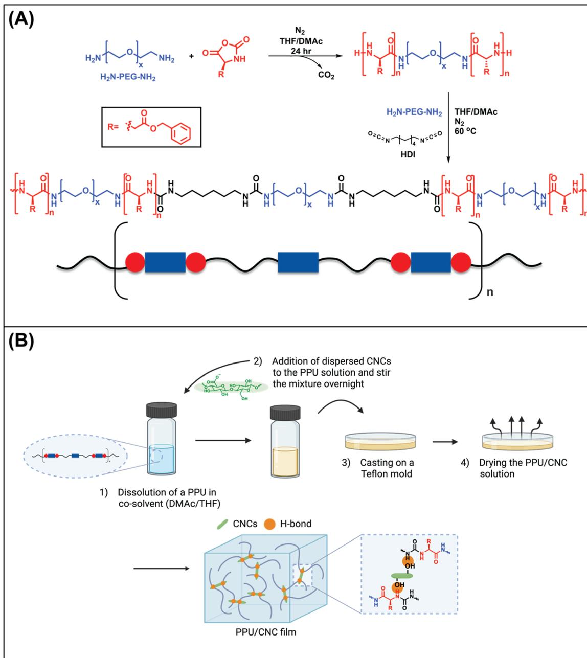
**Fig. 1** (A) Overview of the PPU synthesis process, which is utilized as the matrix material in our nanocomposite system. (B) Step-by-step illustration for the preparation of the PPU/CNC nanocomposite film, highlighting the formation of hydrogen bonding interactions between the PPU and CNCs.
