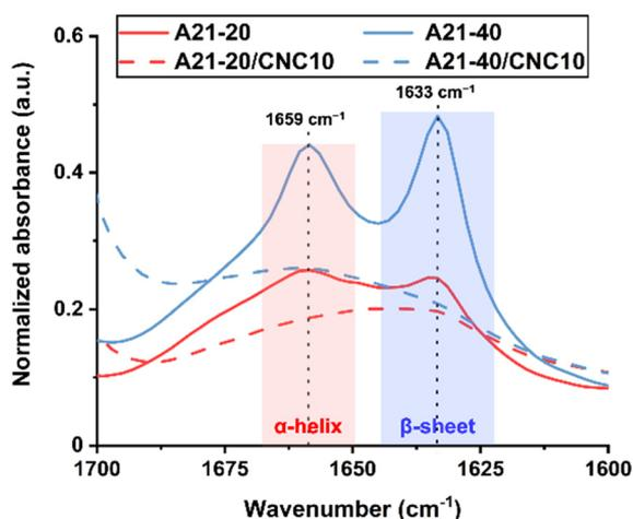
Fig. 2 ATR-FTIR spectra of PPU (solid lines) and PPU/CNC nanocomposites (dash lines) in the amide I region (1700–1600  $\text{cm}^{-1}$ ) to identify peptidic ordering with varying the PBLA and CNC content.
