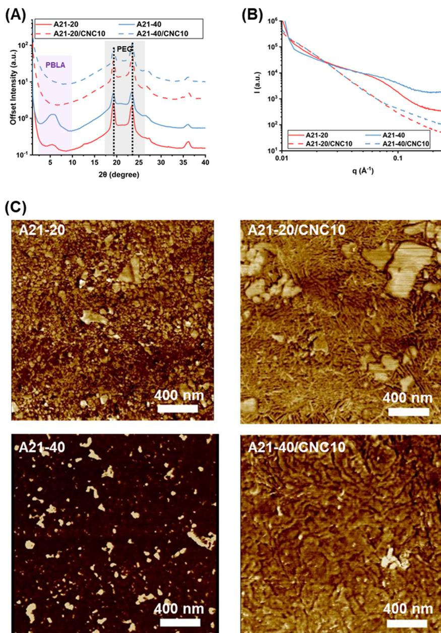
**Fig. 4** Characterization of hierarchical structures of PPU and PPU/CNC nanocomposites from nano- to micro-scale: (A) WAXS data probing the crystallization behavior of the soft phase (*i.e.*, PBLA and PEG segments). (B) 1-D SAXS profiles of PPU and PPU/CNC films with varying PBLA and CNC content. (C) AFM phase images of the surface of dried PPU and PPU/CNC nanocomposite films ( $2 \times 2 \mu\text{m}$ ).
