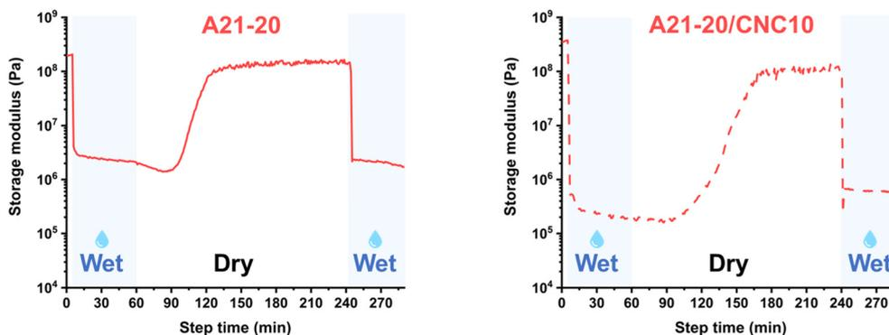
Fig. 7 Representative PPU (A21-20) and PPU/CNC nanocomposites (A21-20/CNC10) showing the reversible variation of the storage modulus during drying–wetting–drying–wetting cycles. Throughout the drying cycle, the films were left to air-dry in ambient air at room temperature for 180 min.
