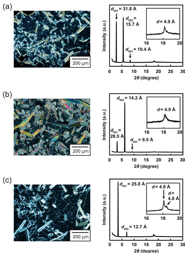
Fig. 2 Polarizing optical micrographs (left panels) and XRD patterns (right panels): (a) compound **1** in the smectic B phase at 30 °C, (b) compound **2** in the smectic B phase at 30 °C, and (c) compound **3** in the smectic phase at 30 °C.
