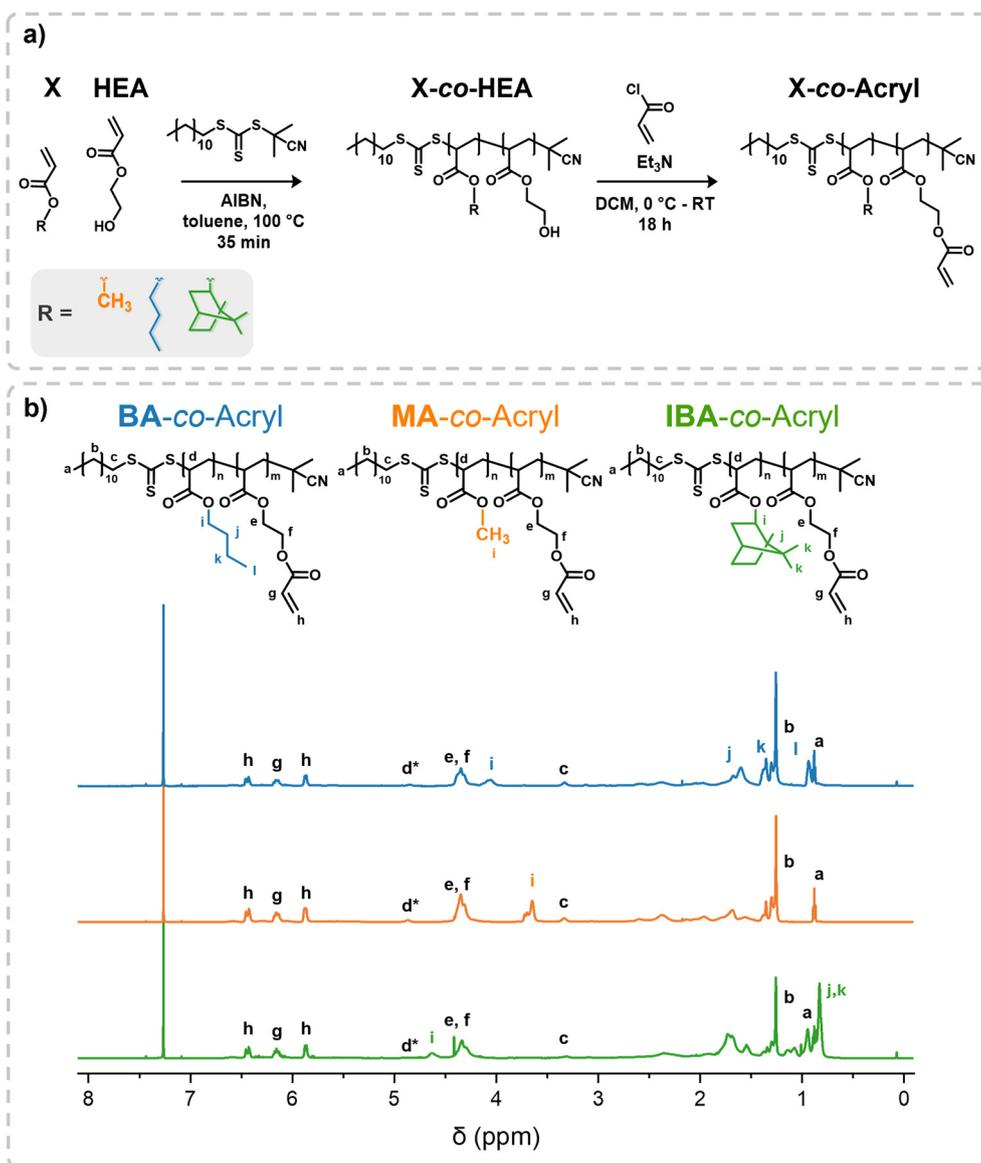
Fig. 1 a) Synthetic pathway for the preparation of each macromolecules using RAFT-controlled radical polymerization followed by functionalization with crosslinkable acrylate groups and b)  $^1\text{H-NMR}$  spectra ( $\text{CDCl}_3$ , 600 MHz, 128 s, 295 K) of BA-co-Acryl (top, blue), MA-co-Acryl (middle, orange) and IBA-co-Acryl (bottom, green) polymers after post functionalization, where  $d^*$  represents the protons of the monomer directly adjacent to the S of the chain transfer agent.
