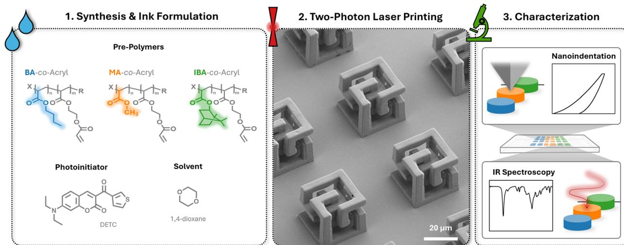
**Scheme 1** Overall approach used to determine the structure–property relationships between three polymer inks BA-*co*-Acryl, MA-*co*-Acryl, and IBA-*co*-Acryl through 1) rational design of copolymer materials for ink formulation, 2) determination of optimum parameters using 2PLP and 3D printing microstructures, and 3) characterization through infrared spectroscopy and nanoindentation to determine chemical and mechanical properties, respectively.
