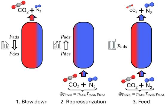
Fig. 1 The 3 steps of the PSA/VSA process model. The colors indicate (not to scale) the concentrations of CO<sub>2</sub> (red) and N<sub>2</sub> (blue) in the gas phase at the end of each step.
