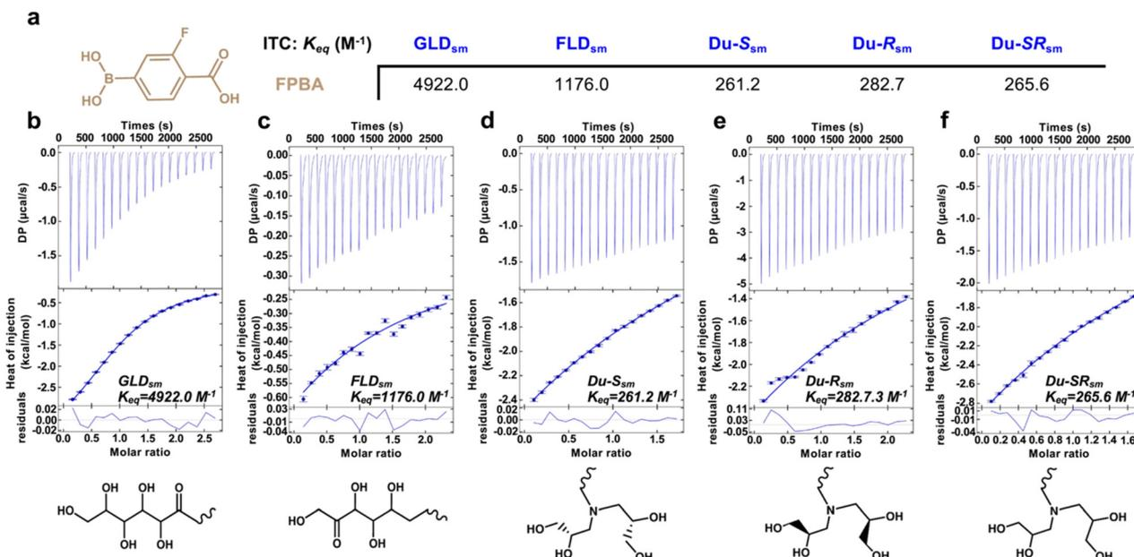
**Fig. 5** Isothermal titration calorimetry (ITC) studies, showing (a) tabulated binding affinities ( $K_{eq}$ ) quantified for binding between small molecule diol derivatives and FPBA, as well as representative model-fit data for binding of diol derivatives (b) GLD<sub>sm</sub>, (c) FLD<sub>sm</sub>, (d) Du-S<sub>sm</sub>, (e) Du-R<sub>sm</sub>, and (f) Du-SR<sub>sm</sub>.
