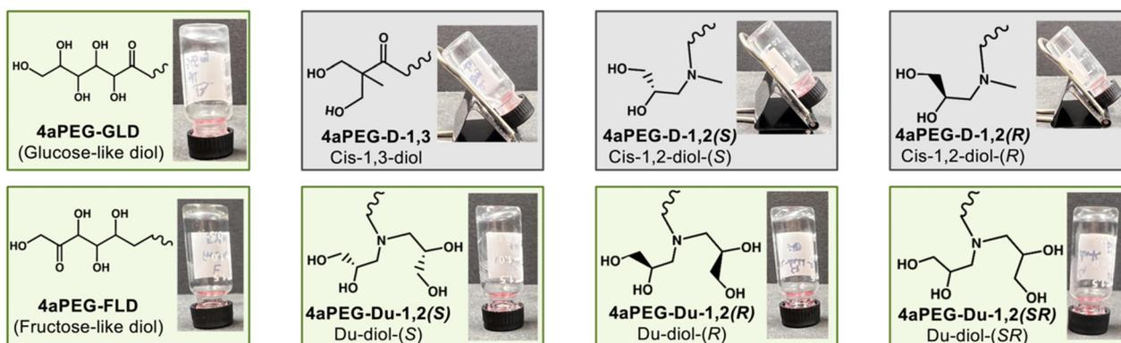
Fig. 2 Hydrogel screening *via* vial inversion of 10% (w/v) mixtures in phosphate buffer (0.1 M, pH 7.4) of 4aPEG-FPBA and different 4aPEG-diols, consisting of 4aPEG-GLD, 4aPEG-FLD, 4aPEG-D-1,3, 4aPEG-D-1,2(S), 4aPEG-D-1,2(R), 4aPEG-Du-1,2(S), 4aPEG-Du-1,2(R), or 4aPEG-Du-1,2(SR). Green boxes indicate samples that formed self-supporting hydrogels.
