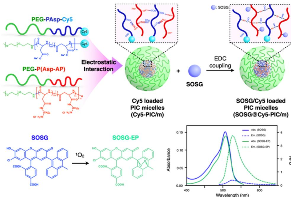
**Fig. 1** Schematic illustration of SOSG/Cy5-labeled PIC micelles (SOSG@Cy5-PIC/m). The conjugated SOSG enables the detection of  $^1\text{O}_2$  by changing its fluorescent characteristic, while the Cy5 constantly reports the position of the probes in biological systems.
