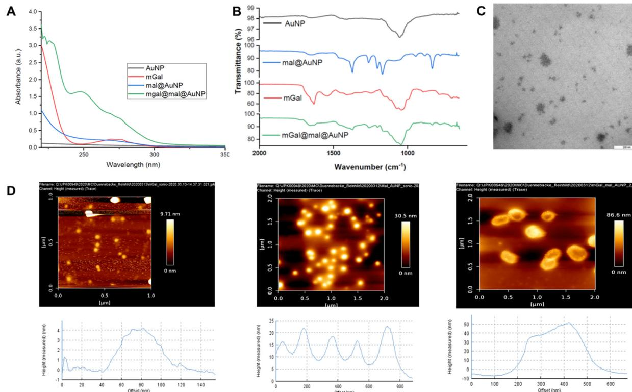
**Fig. 2** Characterization of galectin conjugated nanoparticles. (A) UV spectra of mGal@mal@AuNP show a 280 nm characteristic signal of protein conjugates. (B) IR spectra of mGal@mal@AuNP show prominent characteristics of both mGal and mal@AuNP. (C) TEM images of mGal@mal@AuNP show presence of 50 nm particles and other small particles. (D) AFM images of naked AuNP, mal@AuNP and mGal@mal@AuNP, respectively. The mGal@mal@AuNP show oval shaped structures of size 50 nm.
