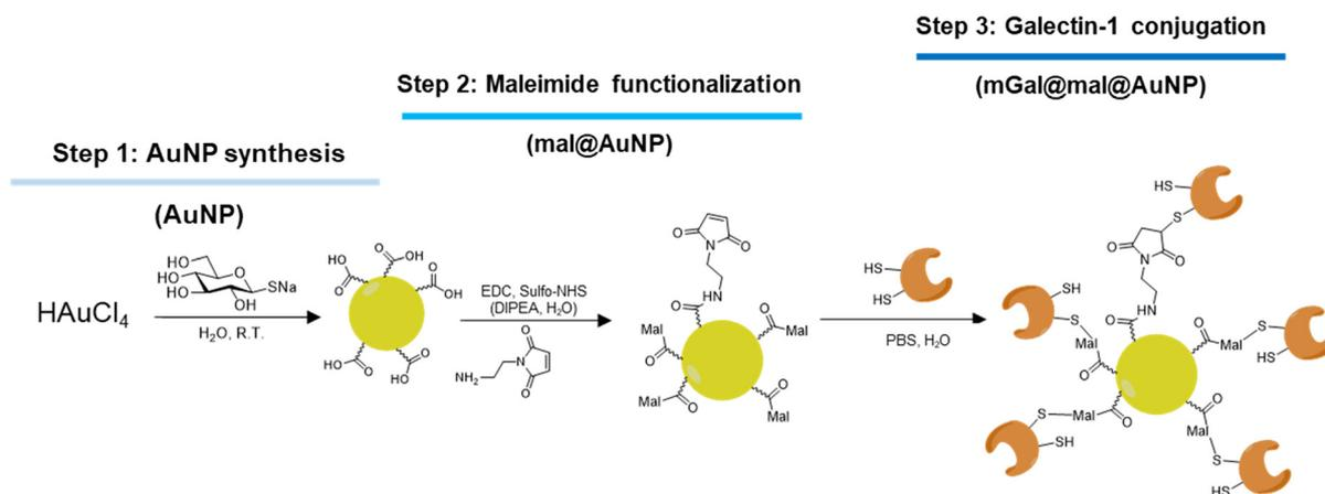
**Fig. 1** Schematic synthesis of galectin-conjugated nanoparticles. Glucose stabilized gold nanoparticles (AuNP) were first functionalized with terminal maleimide groups using amide coupling chemistry (mal@AuNP). Then the galectin was conjugated to the maleimide functionalized gold nanoparticles using thiol maleimide click chemistry to obtain mGal@mal@AuNP.
