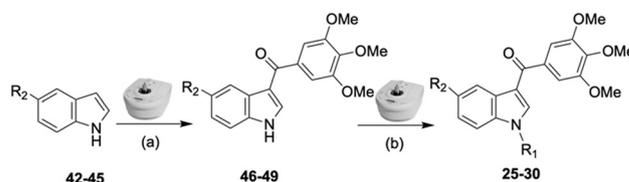
**Scheme 2** Reagents and conditions: (a) 3,4,5-trimethoxybenzoyl chloride, AlCl<sub>3</sub>, 1,2-dichloroethane, MW irradiation (closed vessel, 150 W, 110 °C, 4 min), yield: 41–96%; (b) 2-bromopyridine, 3-bromopyridine or 2-bromopyrimidine, CuI, Cs<sub>2</sub>CO<sub>3</sub>, 1,10-phenanthroline, dry 1,4-dioxane, MW irradiation (closed vessel, 150 W, 180 °C, 40 min), yield: 29–81%.  $R_1$ : see Table 2.  $R_2$ : **42**, **46**: Cl; **43**, **47**: F; **44**, **48**: CN; **45**, **49**: OMe.
