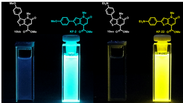
Fig. 3 Fluorescence comparison of 2-aryl and 3-arylthieno[3,2- b ]pyridin-5(4 H )-ones (10 \mu M in CH 2 Cl 2 , excited at 365 nm under a UV lamp).
